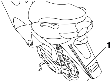
1. Fuel tank breather/overflow hose
