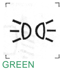
Position (side) lamps ISO 2575 No 433 Colour of tell-tale light: green
