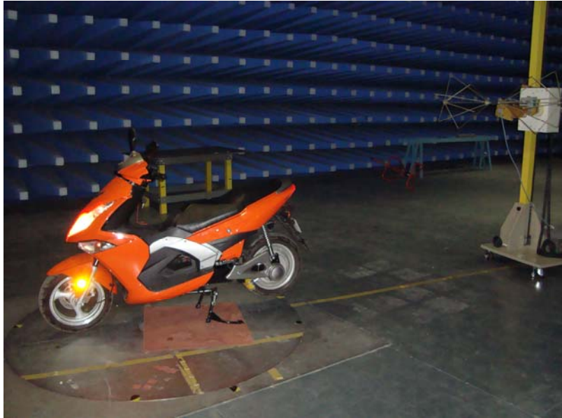
Immunity test status (20MHz to 300MHz)
