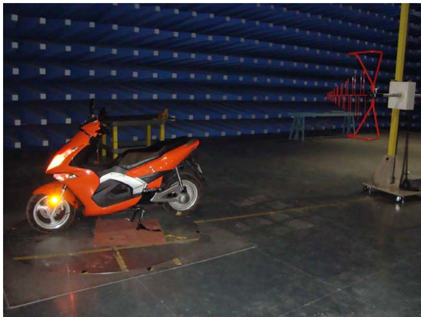
Immunity test status (300MHz to 1000MHz)
