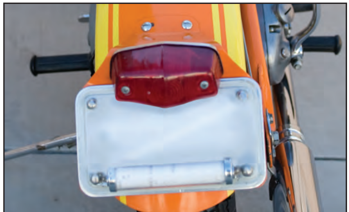
You can see the bolts that hold on the original taillight assembly (below) versus the weld for the newer model (above).
