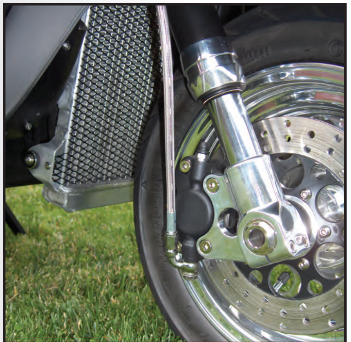
The second radiator hides under the front fender
