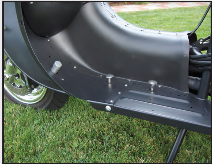
Gary's low-profile shifting mechanism blends in with the original Rabbit design. The button to the far left is the original headlight dimmer switch.
