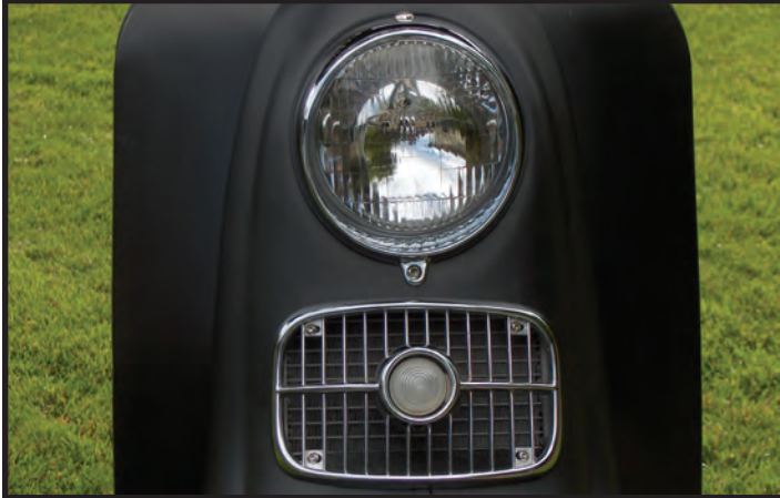
The original grille now provides airflow for the radiator
