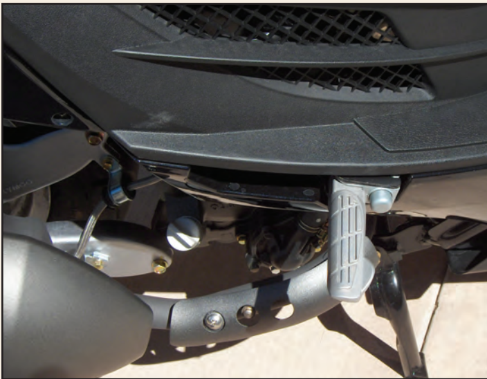
Passenger foot pegs deploy easily with a tap of the foot.
