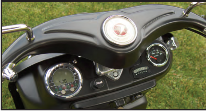
Gary's new gauges fit in with original Rabbit panel. L to R: computer-controlled diagnostic gauge, original choke, battery meter (was gas gauge), radiator gauge (was original gas intake) and new coolant intake.
