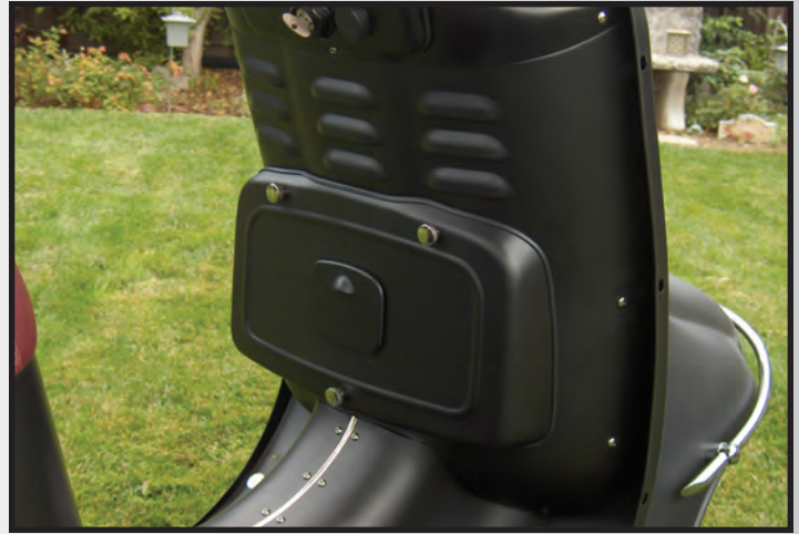
Originally holding the gas tank, the legshield now holds the battery, computer controls and the top radiator.
