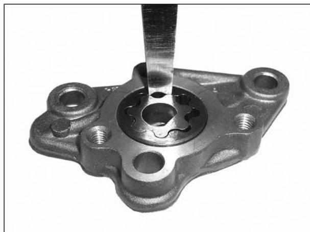
Measure the pump body clearance.
