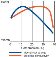
In general, the mechanical strength of the connection is greatest when the total copper cross section area has been reduced by 10%. With less compression (undercrimp) the wire will often slide out of the terminal. With too much compression (overcrimp) the strands of the wire have a tendency to break.
