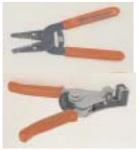
These tools feature ground nests into which wires can be placed for stripping. Whilst useful as service tools they can be easily misused. Success relies on the operator putting the right wire into the right nest. All too often in production this does not happen. Furthermore a large range of tools are required to cover a reasonable wire size range.
