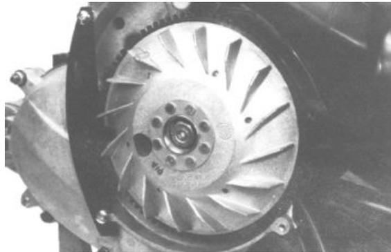
Using the appropriate tool, unscrew the lock-nut of the flywheel.
