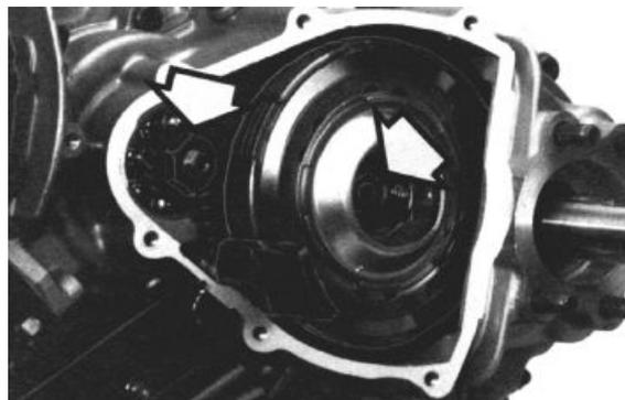
Using the special tool, undo the fixing nut of the clutch assembly
