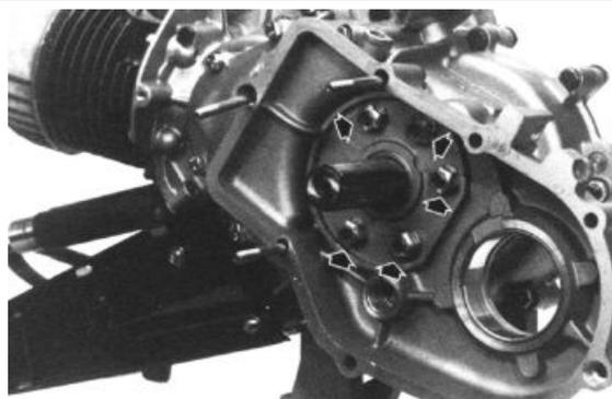
Remove the bearing using a section of tube.
