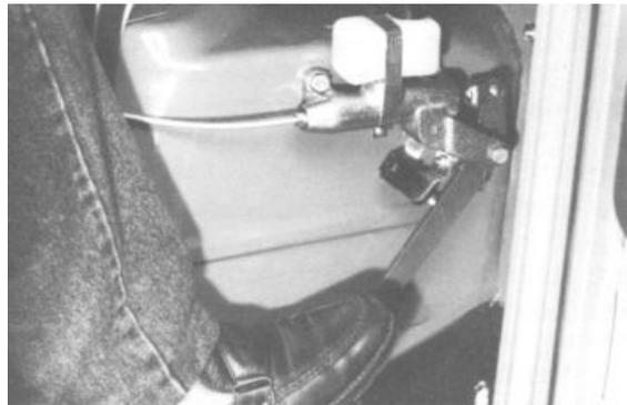
Lower the pedal, keeping it pressed, undo the bleed screw on a rear wheel, let the air out, after this bleed point has been connected through a small rubber pipe to a tray full of brake fluid.
