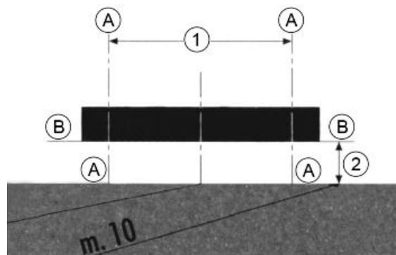
4.If this is not so, adjust the headlight by means of the two screws (1) to correct any beam alterations.
