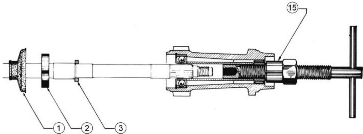
2) - Remove the specific tool from the axle from, add the parts. 9 and 14 as shown in the figure and complete the fitting until the spacer ring touches the ball bearing (3).
