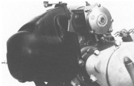
Undo the fixing screws of the cylinder head.
