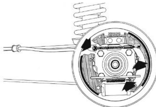
**Brake cylinder and shoe disc**
