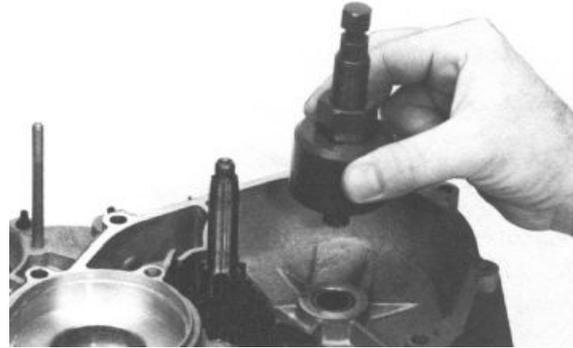
After warming the crankcase, remove it with light taps of the hammer.
