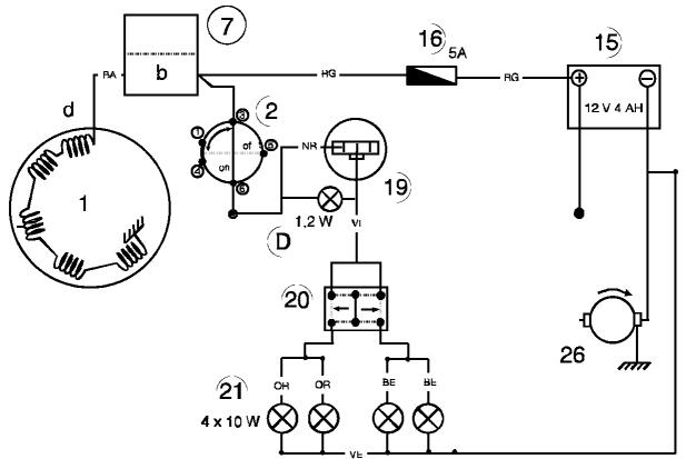
The indicator circuit is supplied by direct current. Having selected the side for the indicator function using the control button (20), the indicator control unit supplies the lamps (21) with an intermittent current.
