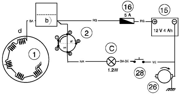
The low oil level telltale circuit is supplied by direct current.
