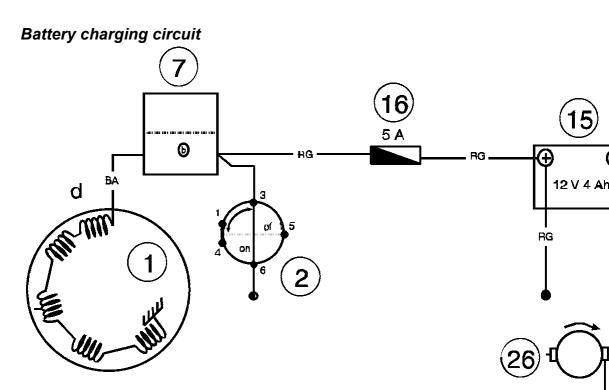
The rectified and regulated current which is given out by the regulator (7) is sent towards the battery through the 5A (16) protection fuse. Once the voltage given out by the regulator is higher than battery voltage, then the battery will start to charge.
