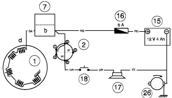
The horn circuit is supplied by direct current.
