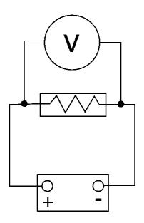
This enables the voltage to be checked. It is connected up in parallel on the component to be checked. Two types of voltmeter are available, one for alternating current and one for direct current.
