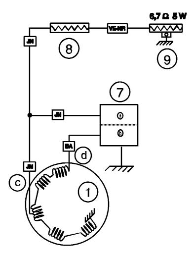
The choke circuit is fed by the alternating current circuit limited in voltage. The heat expandable component (8) is thus supplied only when the motor is working. The latter is supplied through a limitation resistance (9), in this case 6.7  $\Omega$  5 W which limits the amount of current passing through the heat expandable component.
