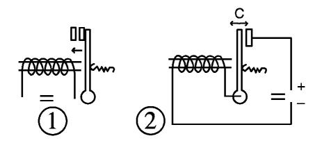
Relay: by passing a direct current through the coil in the relay, the magnetic field thus created attracts the contact blade of the relay which makes contact with the outlet terminal.
