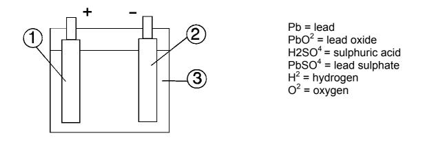
Chemical reaction:  $PbO^2 + H2SO^4 + Pb = H^2 + O^2 + PbSO^4$
