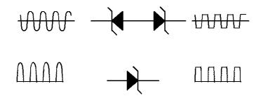
In order to limit maximum voltage, for instance in a lighting circuit, a zener diode is used. This system can be used either with alternating current or rectified current.
