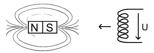
A magnet produces a magnetic field oriented from the north to the south of the magnet. If a coil is brought into proximity with this magnetic field, then an induced voltage V will be produced in the coil.
