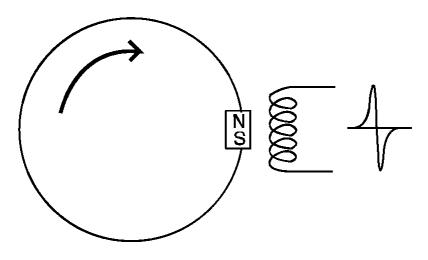
When the magnetised mark passes in front of the coil in the sensor, this creates an induced current in the coil which is used by the system to determine the position of the magnet.
