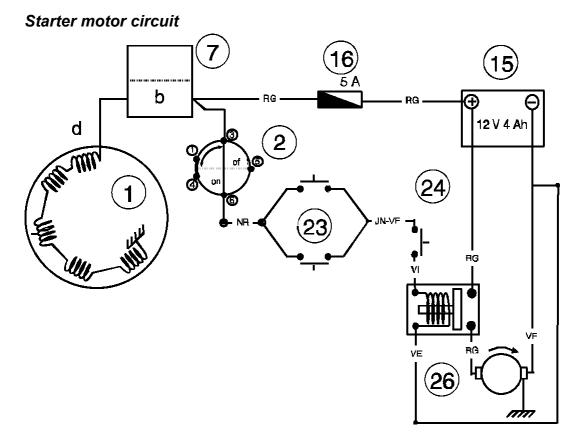
The starter motor is supplied by the battery, which must thus be sufficiently charged in order to allow it to operate. The starter motor is the biggest consumer of current on the vehicle. Furthermore, frequent use of the starter motor on a vehicle which does not do a lot of mileage will rapidly lead to complete discharging of the battery.
