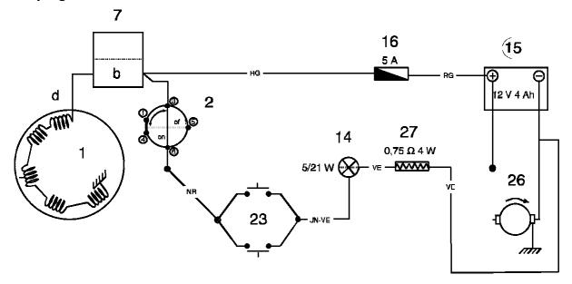
The stop light circuit is supplied by a direct current.
