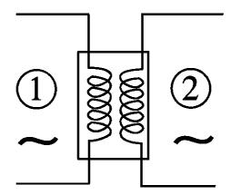
The current passing through coil n°. 1 creates a magnetic field, which acting on coil n°. 2 creates an induced electric current in the latter.
