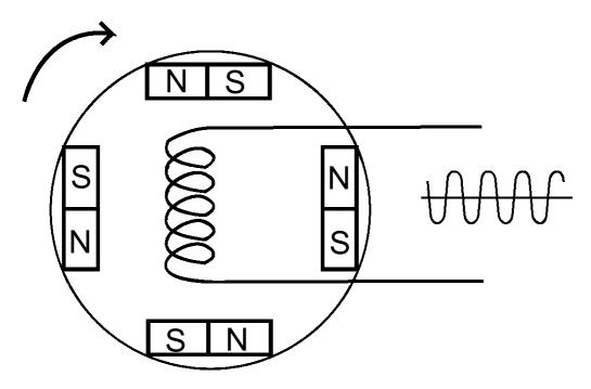
The rotation of magnets around the coil create an induced current in the latter. This current can be used to supply an electric circuit.
