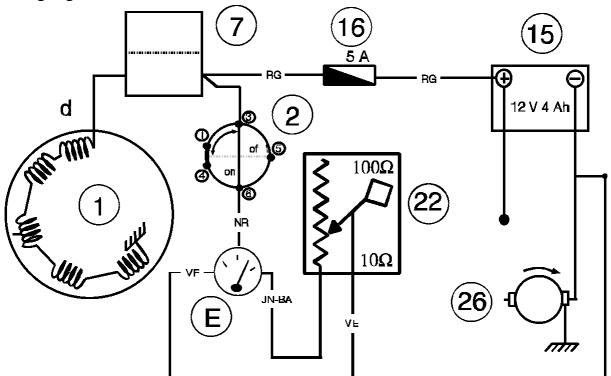
The fuel gauge circuit is supplied with a direct current.
