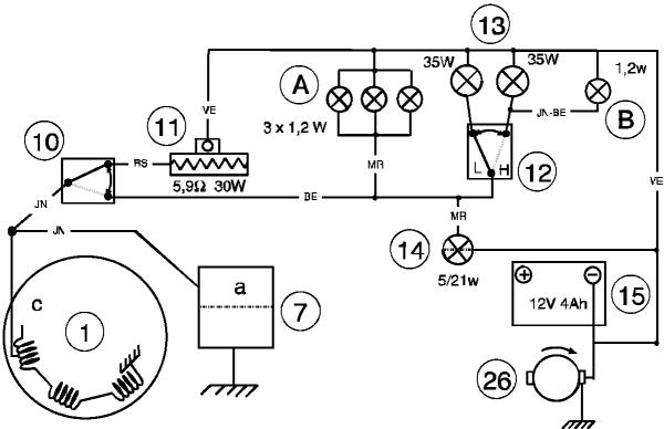
The lighting circuit is fed by the alternating current circuit limited in voltage. In the event that the lighting is not used, the current produced by the lighting coil must be destroyed so as not to burn out the coil. This current is thus directed towards the resistance (11) where it will be consumed.
