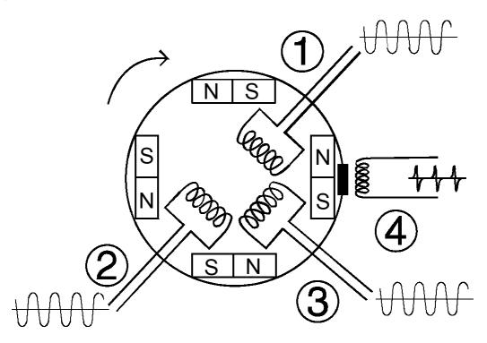
A flywheel consists of a rotor (a group of magnets mounted onto a rotating support) and a stator (a group of coils). When the rotor rotates around the coils, this produces alternating current in the coils.
