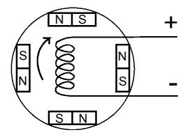
The passage of direct current through the coil creates a magnetic field which opposes the field of the magnets thus causing the coil to rotate.
