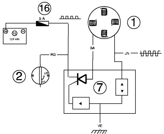
Two supply circuits exist: one circuit with alternating current limited in voltage for lighting, the choke etc., and one circuit with rectified and regulated current for battery charging, ignition etc....
