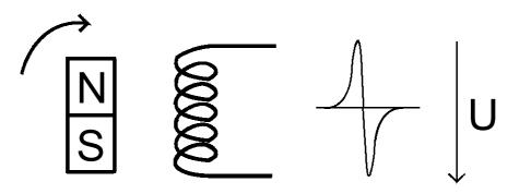
If a magnet is rotated next to a coil, then an induced alternating voltage is created within the coil, the value of which depends on the intensity of the magnetic field and the frequency of which depends on the speed of rotation of the magnet. The higher the speed of rotation of the magnet, the greater the electrical voltage in the coil.
