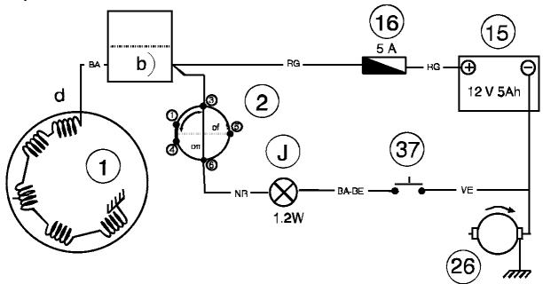
The oil pressure telltale circuit is supplied by direct current.
