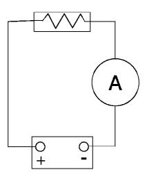
This enables current to be measured. It is connected up in series on the component to be checked.
