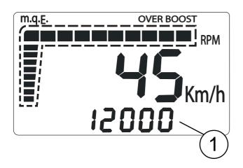
When the engine speed exceeds the maximum limit, "OVER BOOST" is displayed on top of the screen.
