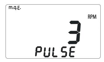
Pressing the control button for more than 3s will allow you to set the number pulses per engine revolution.
