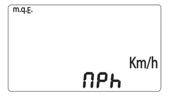
Pressing the control button for more than 3s will allow you to set the unit of measurement.
