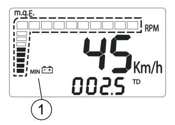
The battery charge telltale blinks if the battery's voltage goes below 9 volts and it stops blinking when the voltage goes back over 9.5 volts.
