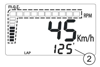
Display (2) of hours and minutes when the time is more than 1 hour.
