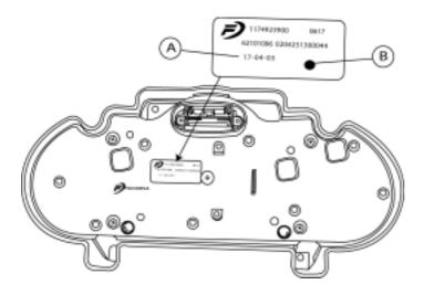
Identification of the new instrument clusters: On the back of the cluster on the label, For the Elystar 50cc
