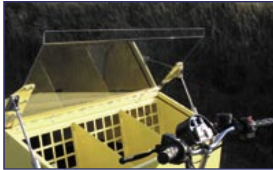
The weather protection in the up position functions as a windbreak for the driver.
