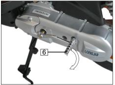
CAUTION After starting the engine, check that the kick starter lever (6) is returned to its normal position. - Propping up the scooter when operating the kick starter.
