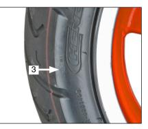
Recommended minimum profile depth: 2.0 mm Observe the wear marks (3).
