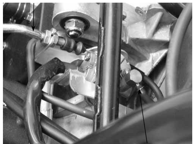
Oil Outlet Line
