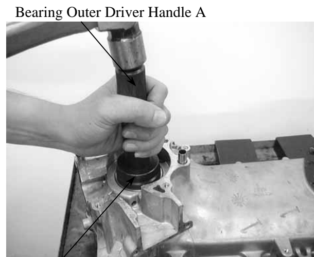
Bearing Outer Driver Handle A Bearing Outer Driver, 42x47mm Pilot, 20mm
