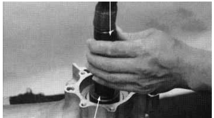
Bearing Outer Driver, 42x47mm Pilot, 20mm
