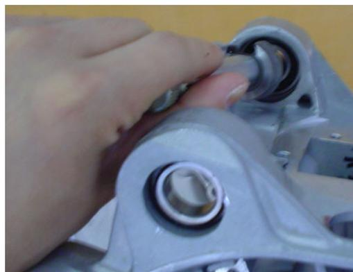
**Install crankshaft bearing**
