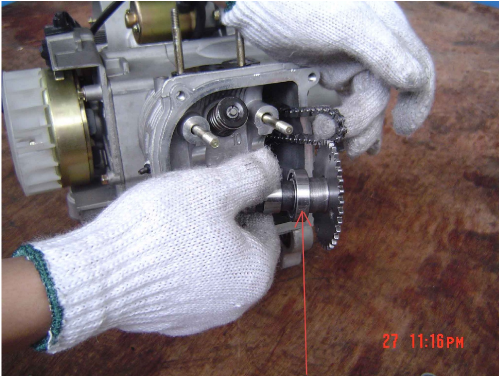
Fig. 8. Install the camshaft.
