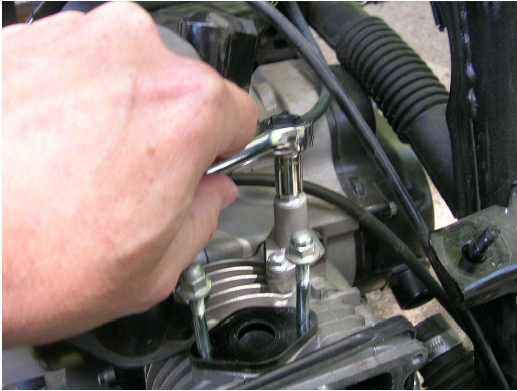
Fig. 8. Remove the chain regulator
