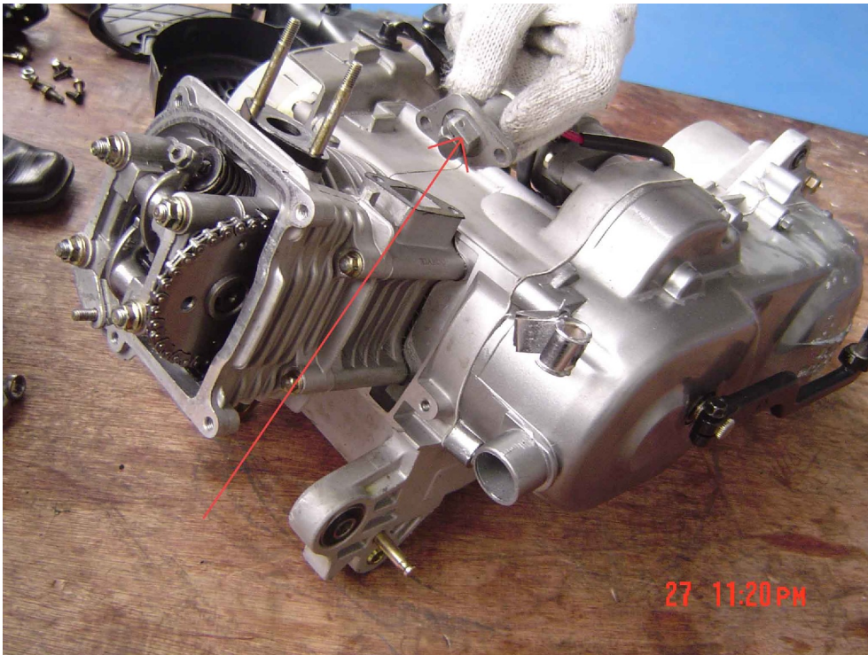
Fig. 12. Install chain tension assembly.
