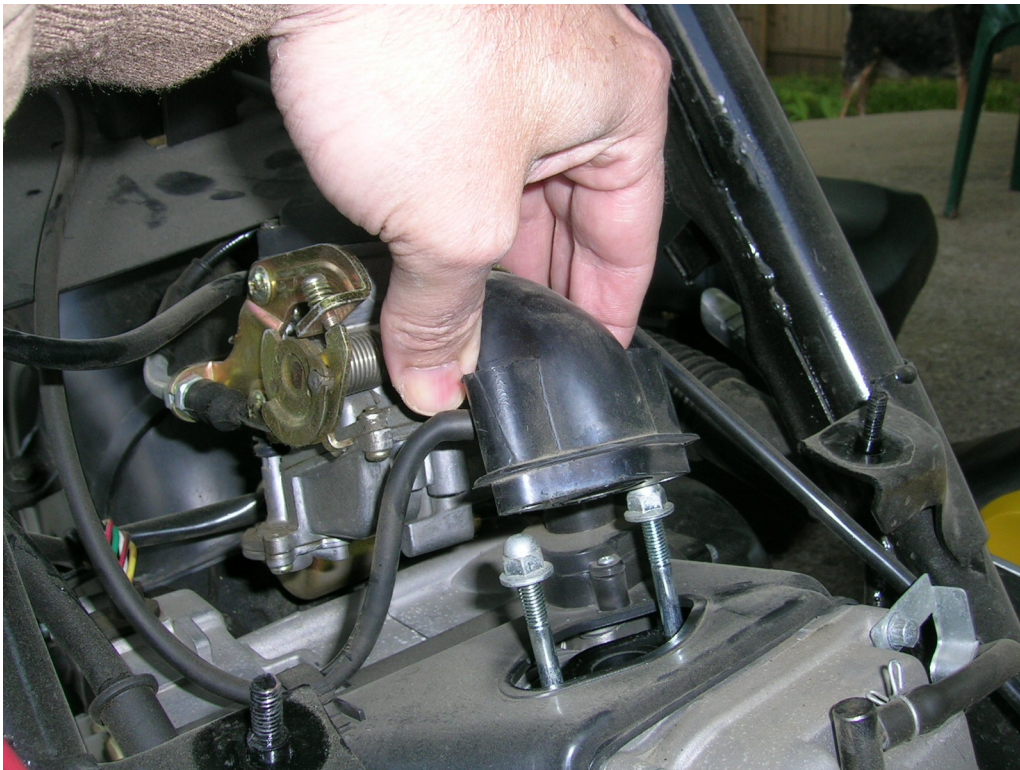
Fig. 3. Remove carb inlet tube.
