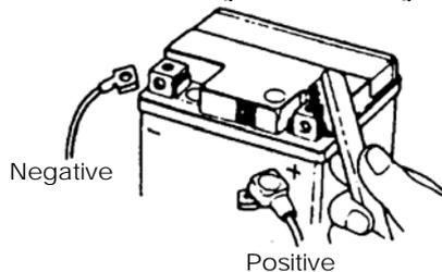
Remove the battery terminals and clean if there are dirt and corrosion on them.
