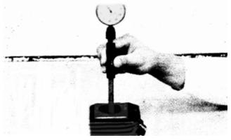
Calculate the piston-to-cylinder clearance.
