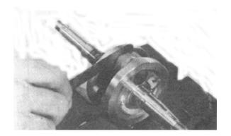
Measure the connecting rod big end radial clearance at two different point across from each other.
