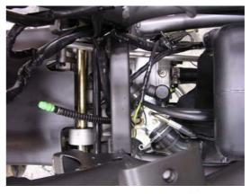
Adjust the clearance of the throttle valve cable.
