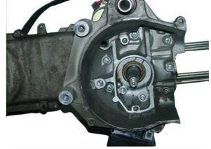
Remove the right crankcase from the left crankcase by using a pulley.
