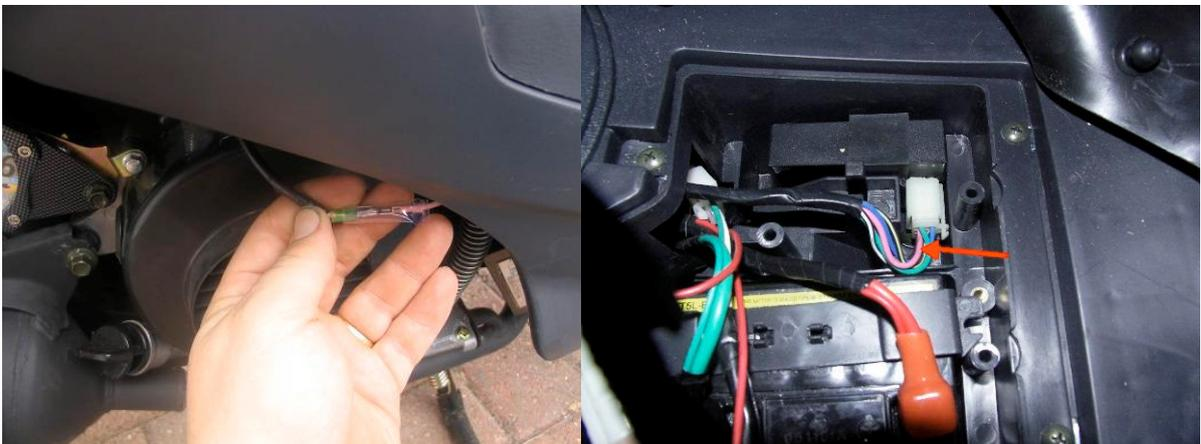
When you have disconnected this wire you will need to cover the ends with the electrical tape. **DO NOT DISCONNECT ANY OTHER WIRE.** The pink wire sends information about the speed of the back wheel to the CDI unit. If the CDI unit doesn't receive this info (because we disconnected it!) it thinks you are not moving and will allow the engine to go to full throttle.
