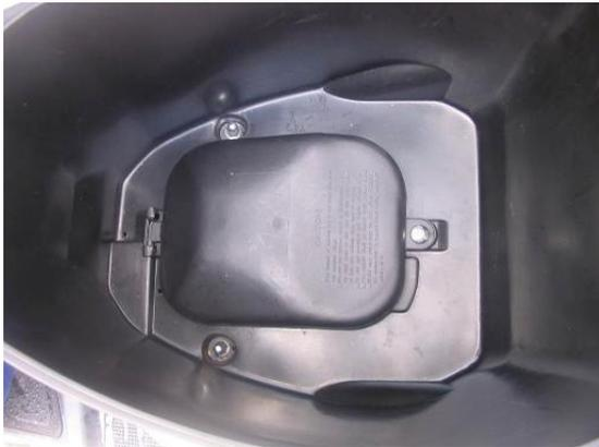
Opening this cover by removing the silver screw will give you access to the Carburettor.
