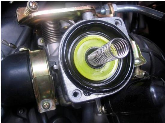
Now Carefully remove the rubber seal and the yellow disc will come with it. Inside this part there is a white plastic 'Plug' and a metal needle two small washers on it. One is loose and will fall off never to be seen again, if your not careful, and the other is fixed to the pin in a groove at the top. There should also be a small rubber
