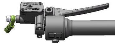
The front brake grip is located on the right handle. Grasp the grip in the direction of the handle to make the front wheel brake.
