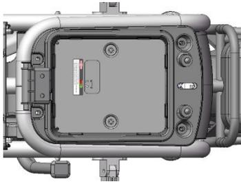
Use the bucket key to open the bucket and make sure the main power switch is in the ON position.
