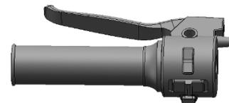
The rear brake grip is located on the left handle, and grasp the grip in the direction of the handle to make the rear wheel brake.
