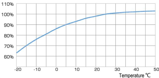
**Capacity Retention Characteristics**
