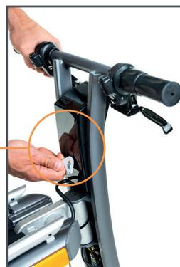
To turn off the Stigo scooter after use, press and hold down the ON/OFF button for 2 seconds until the display switches off.
