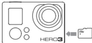
1. Slide memory card into card slot with label facing front of camera.
