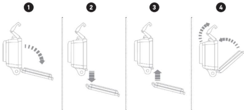
1. Open the backdoor of the housing so that it is hanging downwards.
