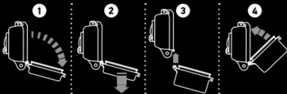
1. Open the backdoor of the housing so that it is hanging downwards.
