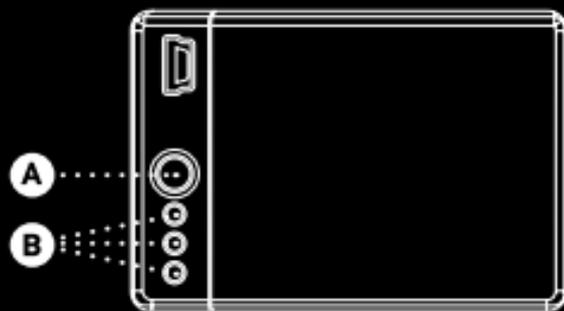
1. Press the BacPac button (A) once and the LED lights (B) will illuminate to indicate power level.
