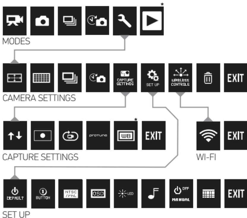
**\*Note: White Balance and Playback** only appear in your camera display if **Protune™** mode is turned **ON** or **Playback** is activated.
