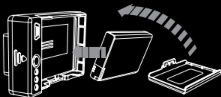
3. To insert the battery, align battery as illustrated and push into place.
