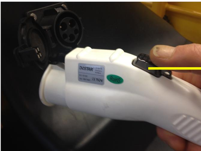
PRESS BUTTON AND PUSH MALE CHARGING PLUG INTO FEMALE CHARGING PLUG
