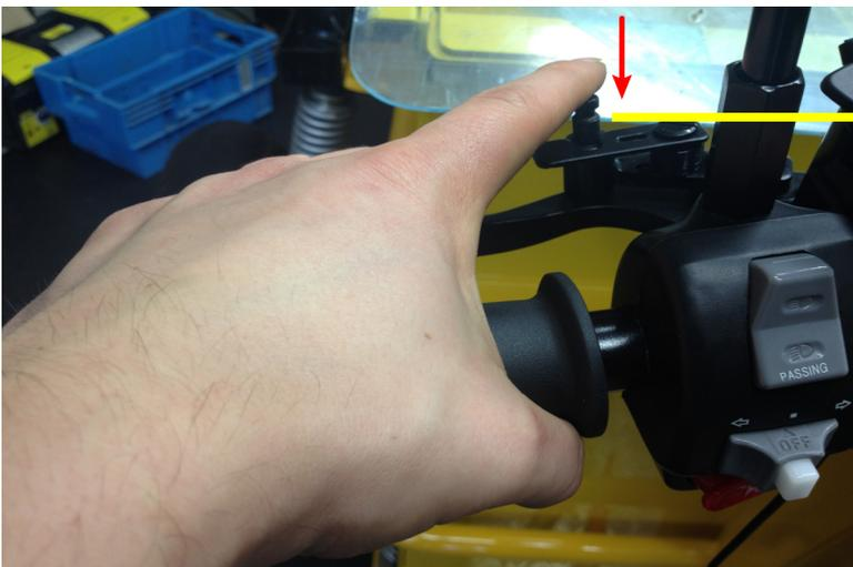
ACTIVATE LEFT PARKING BREAK BY PRESSING THE HANDLE AND THEN PUSH THE PIN DOWNWARD
