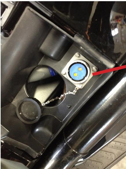
Charging plug with removed protection cup.
