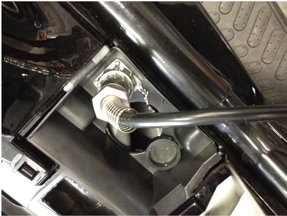
Charger is connected to scooters charging plug.
