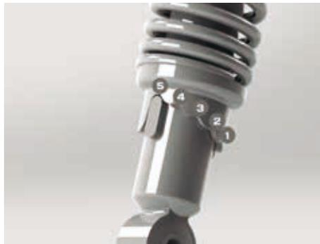
*Pre-load levels: 5. Minimum pre-load - 1. Maximum pre-load.*
