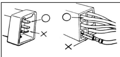
The connector shall be fully inserted in place.
