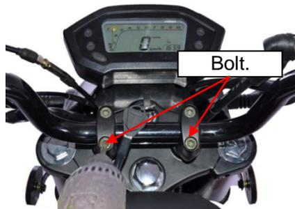
**To install the control subassembly**
