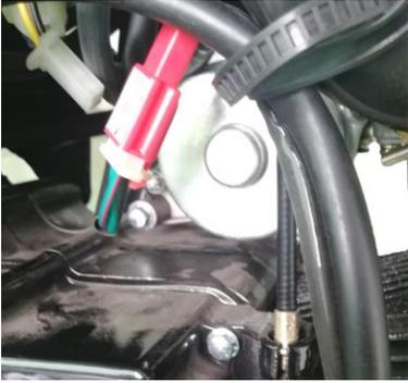
2. Dismantle rectifier bolt and measure two yellow wire whether is short circuit or broken circuit by millimeter.
