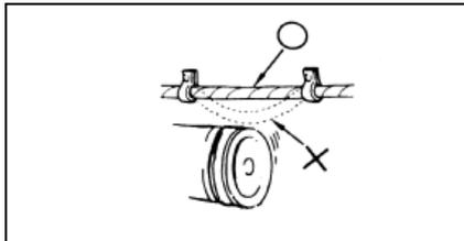
The wire harness shall be clamped at the position without contacting a part that generates high temperature.
