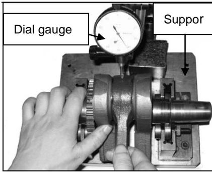
4. Measure the connecting rod large end side clearance, the maintenance limit:  $\leq 0.80\text{mm}$ .
