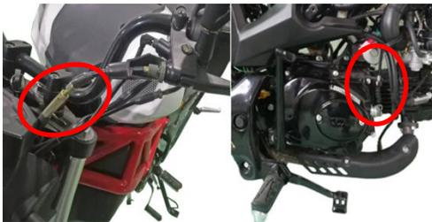
4. Remove engine cycle tube
