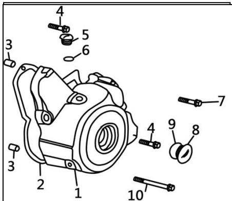
**Disassembly and assembly of left front cover**
