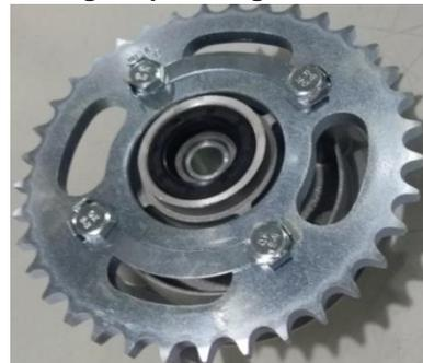
Take out bush and dismantle bolt of rear driven chain disc.
