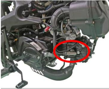
4. Unclamp the inlet pipe clip and remove the cylinder head hanging bolt.
