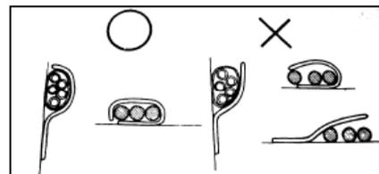
In case of a welded clamp, it shall not bite the wire harness towards the weld mark
