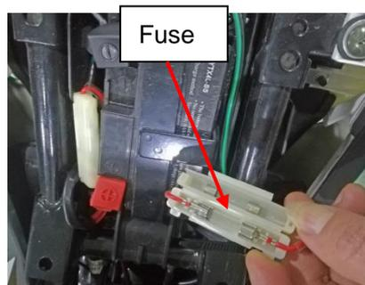
If the new fuse tube is broken again as soon as it is fitted on, it means that somewhere of the electric parts is shorted unexpectedly.
