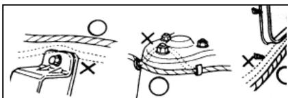
The wire harness shall not be slackened or be forcibly pulled.
