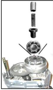
6. Assemble the right crankcase cover by turning the clutch push rod until its rack side faces the crankshaft. (See "Installation of right crankcase cover").
