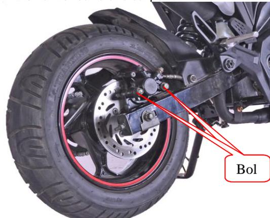
2. Operating brake, if the wears limit line of the brake shoe touch to the side of the brake disc. It shows that the brake shoe has touched the wear limit.
