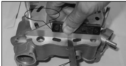
Measure the valve guide aperture.
