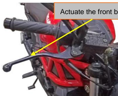
5. When the vacuum pump has fully exhausted the air inside the brake caliper, after the brake fluid is pumped out, firmly nip the handle or completely push down quickly screw the deflating valve bolt, with the torque being (7-9 ) N.m.
