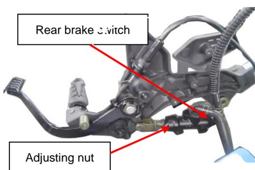
While installing, the wiring of the rear brake lamp shall be in strict accordance with the wiring diagram, and replace the buckle strip
