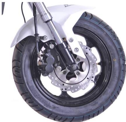
Take out the front wheel. Lift the front fork as high as possible while taking out the front wheel, to avoid damaging the front mudguard.
