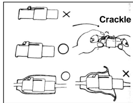
11. Before connecting a connector, make sure the sleeve is not broken and the opening of the intermediate terminal is not too large
