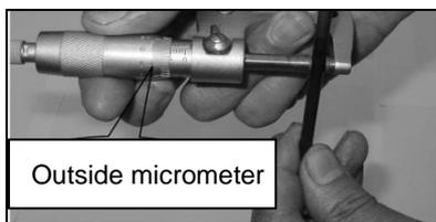
Measure the width of the valve contacting surface.
