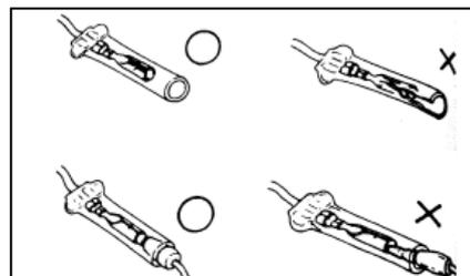
12. The harness fixing strap shall firmly button the specified position on the frame.
