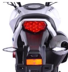
11. Check tail lamp and brake lamp socket whether lose contact or bulb is burned
