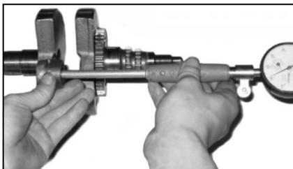
1. Check whether the crankshaft journals are abnormally worn, whether the connecting rod can rotate flexibly and whether there is significant noise while rotating.
