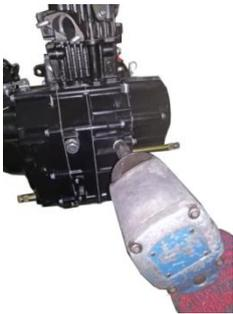
5. Remove the cylinder bolt and washer.
