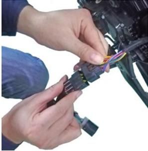
12. Take off ignition switch socket to check whether current input headlamp switch
