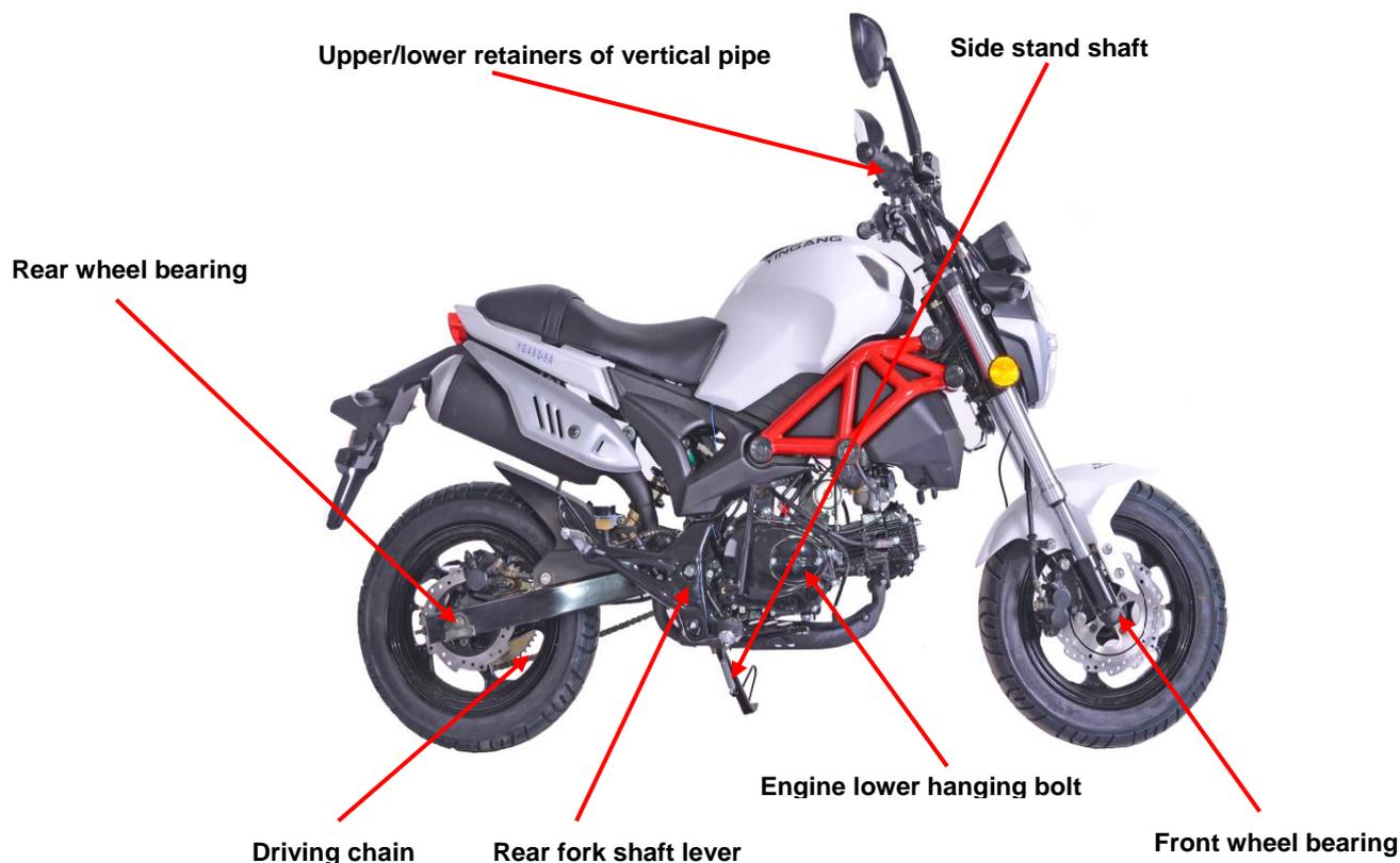
Among the positions shown in the above diagram, besides applying dedicated lubricating oil for chain
