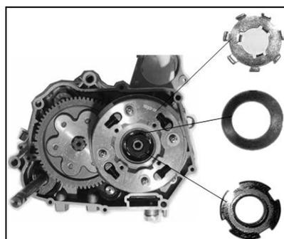
5. Mount the clutch push rod with the clutch push rod
