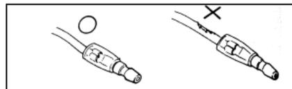
While mounting parts and components, do not press the wire harness.
