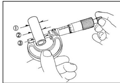
Measure the piston pin hole inside diameter.
