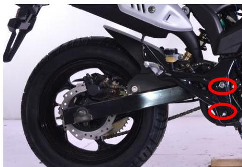
3. Remove the rear damper and rear fork connecting bolt.
