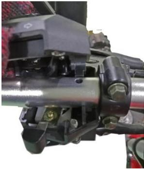
13. Dismantle after brake lamp switch to check it whether lose contact.
