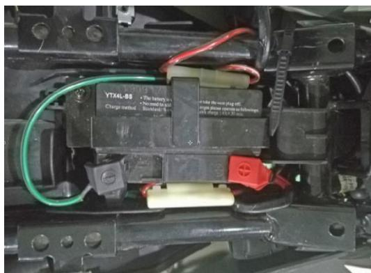
Remove the negative, then the positive pole of the accumulator; unscrew and remove the loosen battery strap
