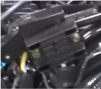
3. Open left cover to check magneto coil whether is burned or loose.
