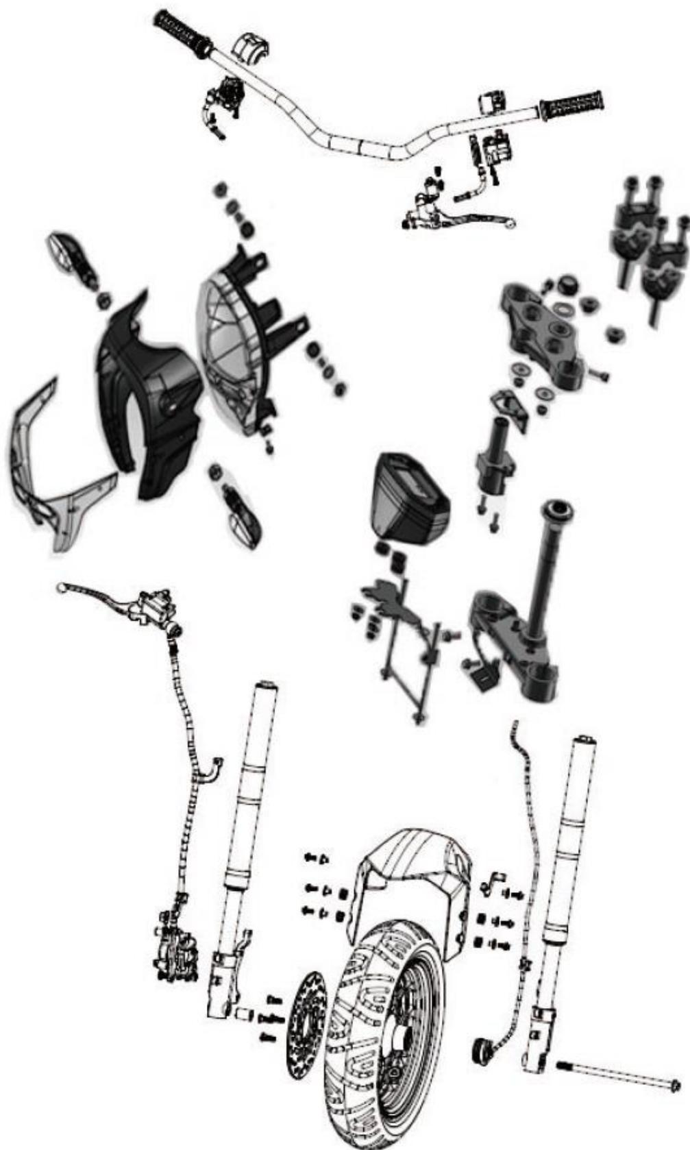
**Front wheel, front suspension device and steering stem**
