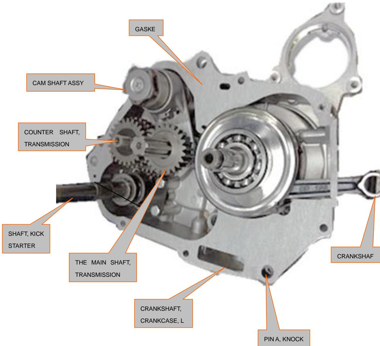
**Crankcase, crankshaft and Shift mechanism**
