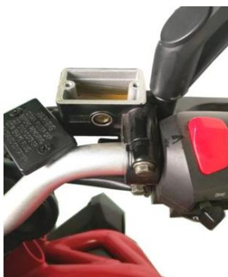
3. Actuate the brake handle, exhaust the air in the dead corner of the brake caliper.
