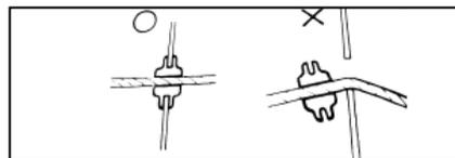
Do not damage the garnish of the wire harness.
