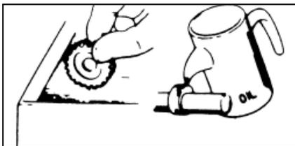
To clean the spare parts, use only the cleaning fluid that is incombustible or has high ignition point. Before reassembling, apply the specified lubricating oil to the sliding surface of the parts and components.
