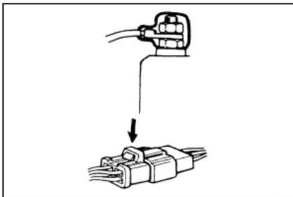
10. While disassembling a connector joints with lock, release the lock before proceeding with operation.
