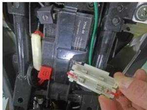
6. Check positive and negative pole of battery whether contact well
