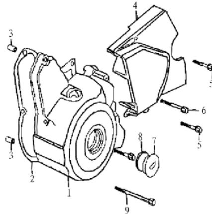
7. Connect the phase sensor and mount the eyehole cover and upper eyehole cover in turn.
