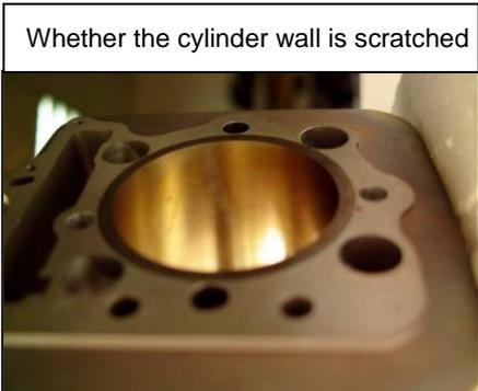
Check the cylinder wall for deformation, and use the edge ruler and clearance gauge to inspect the planeness of the cylinder's joining surface.
