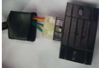
7. check connector socket of rectifier and measure output voltage by multimeter to (13.0-13.3)v
