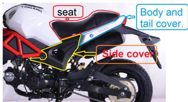
⚠ Notice: Please first Removal of fuel tank(reference Removal and installation of fuel tank , Disassemble step.), Remove side cover.
