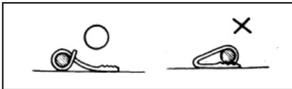
The wire harness shall be clamped at the position without contacting a rotating part or a removing element.
