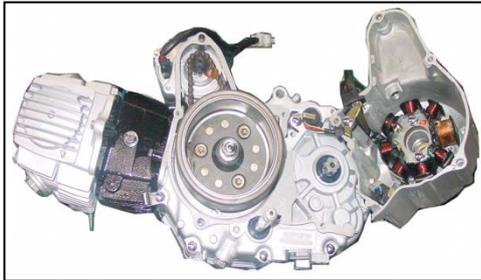
3. Use the rotor fastening tool
