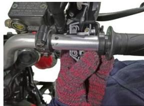
Check steering signal indication lamp socket whether lose contact or bulb is burned
