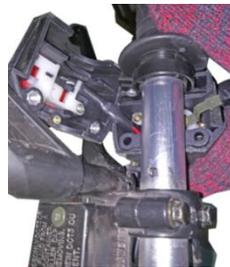
12. Check switch plug of relay whether is loose.
