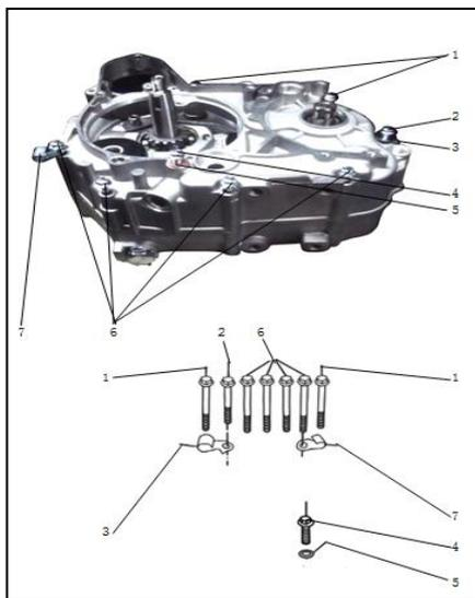
**Removal and installation of crankcase**
