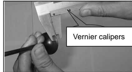
Measure the free length of the valve spring
