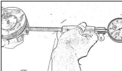
Measure the clearance between the piston ring and the piston groove before removing the piston ring.
