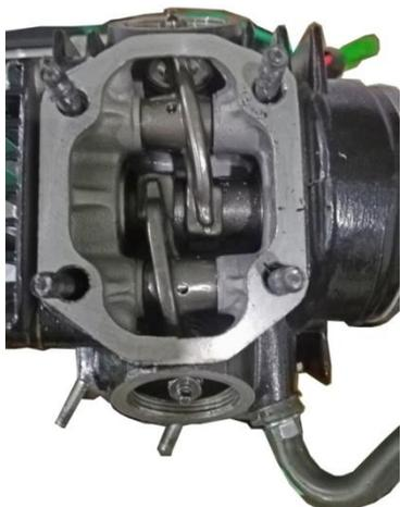
4. After properly timing, pull off the tensioner locking key and coat the mixture of engine oil and molybdenum disulfide on the tensioner to make it tensioned; mount the sprocket retaining plate and retaining bolt
