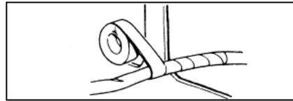
In case of a wire harness with garland, it shall be reliably harnessed.
