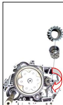
3. Mount the butterfly washer and retaining nut M18. Note to assemble with the protruding side of the butterfly nut washer facing outside.
