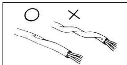
14. When wiring, note when turning it leftwards or rightwards to the limit position, the wire harness shall not be tightened up or slackened, and make sure there is no significant bending, pressing, intervening of marginal parts.
