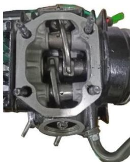
3. Remove the camshaft end cover, loosen the screw and washer at the tail end of the tensioner; turn the screw clockwise with the tensioner locking key so that the tensioner is loosened and locked.
