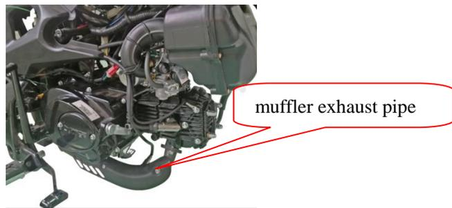
2. Remove the engine cycle tube
