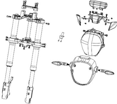
6. Take off meter to check odometer, tachometer and fuel meter whether are damaged.
