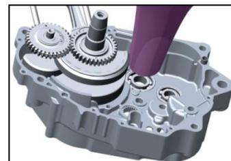
**Removal and installation of driving shaft and driven shaft and gearshift drumand shifting shaft**
