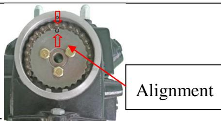
7. Strip the timing chain from the timing driven sprocket, and remove the timing driven sprocket.
