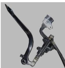
Pull out and pull off the patch plug of the rear brake lamp switch, and carefully pull out the rear brake lamp switch wire and remove the rear brake spring.
