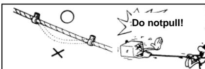
If the wire harness has to contact the edge or sharp corner parts, the contacting part shall be protected with
