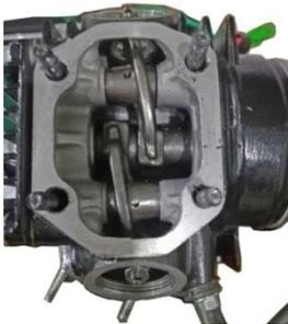
6. Remove the cylinder head and cylinder head gasket.
