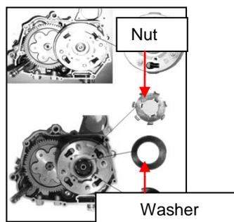
4. Use the fastening tool **5 TOOL** to amp the primary driving and driven gear, and screw up the retaining nut M18 to the tightening torque of 120N.m.
