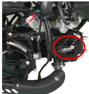
9. Remove the gear shift pedal and left rear cover.
