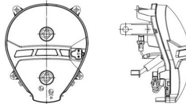
8. Take off remote, near lamp of headlamp and overtake lamp wire to check whether there are current or is loose.
