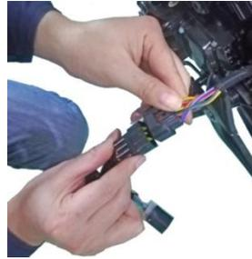
9. Check electrical starting switch whether contact well.
