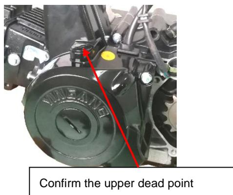
Turn the nut of the flywheel clockwise until the engraved "T" mark on the flywheel aligns with the engraved line on
