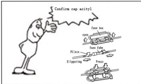
9. The caps must be securely put on the terminals after the operation is complete
