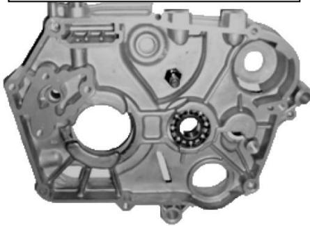
3. Use a Bakelite hammer or a nylon hammer to strike the left hand crankcase gently to separate it with the right hand crankcase.
