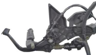
14. Dismantle brake switch before to check it whether lose contact.
