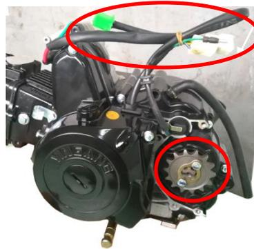
7. Remove the left rear cover of the box and the control mechanism of the variable speed pedal..
