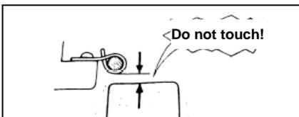
The wire harness shall be clamped at the position without contacting the edge or sharp corners of the vehicle body.
