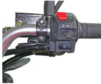
6. Dismantle headlamp bolt to check lamp case whether is damaged.
