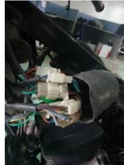
Turn on signal indication switch left handle to check switch whether is rusted or lose contact.
