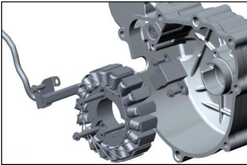
5. Dismantle starting clutch and replace magnetic case.
