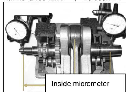
2. Measure the crankshaft radial run out.
