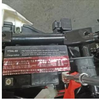
6. Check plate electrode whether is damaged
