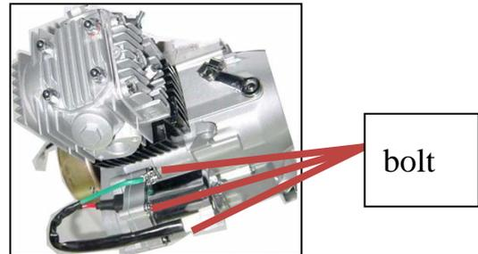
6. Remove the starting sprocket limit plate, remove the transmission chain and drive chain wheel
