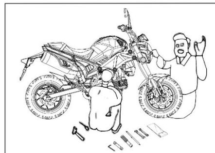
7. Before operating, always remove the negative (-) end of the battery first and take care to prevent the wrench or the like from touching the frame. After operating, reconfirm all the connections, fixings and junctions. If the battery is already removed, connect the positive (+) end first.
