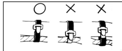
13. The clamp shall reliably bite the wire harness
