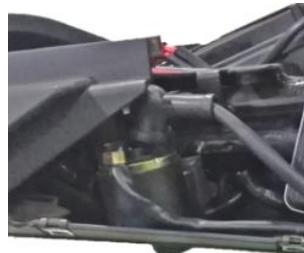
13. Check clutch electrical starting switch plug whether is damaged or loos
