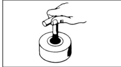
5. The specified or equivalent lubricating grease (oil) must be applied to or refilled into the specified locations.
