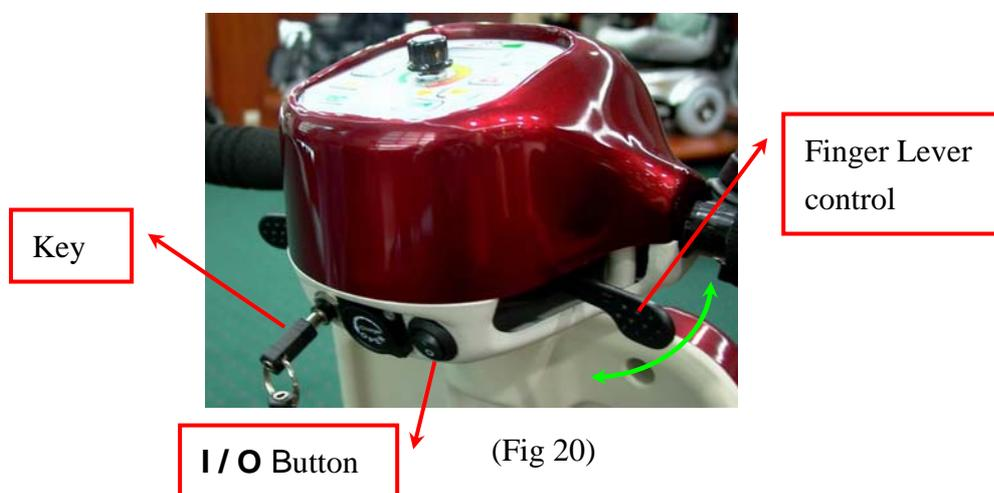
Returning of the finger lever control to its neutral position,(center), will reduce the speed and stop the vehicle by automatically applying the electromagnetic brakes.
