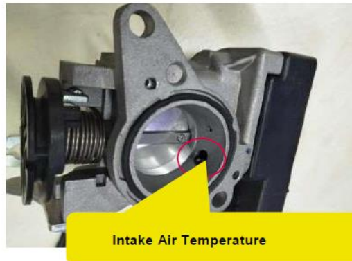
FIG. 4: Intake Air Temperature Sensor
