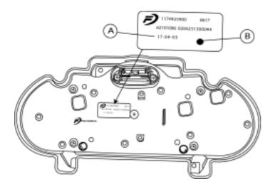
Identification of the new instrument clusters: On the back of the cluster on the label,
