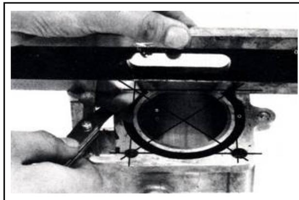
Measure clearance between piston rings and grooves.
