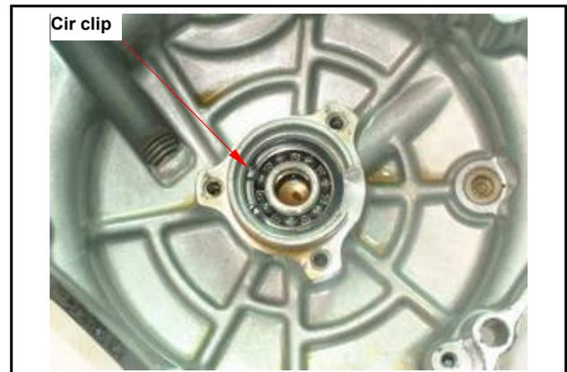
Remove the bearing 6201 with inner bearing puller.
