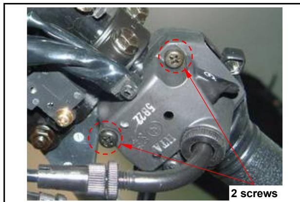
Remove throttle holder, handle switch, cables and grip.
