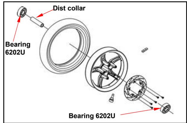
Install the brake disk and then tighten the bolts.
