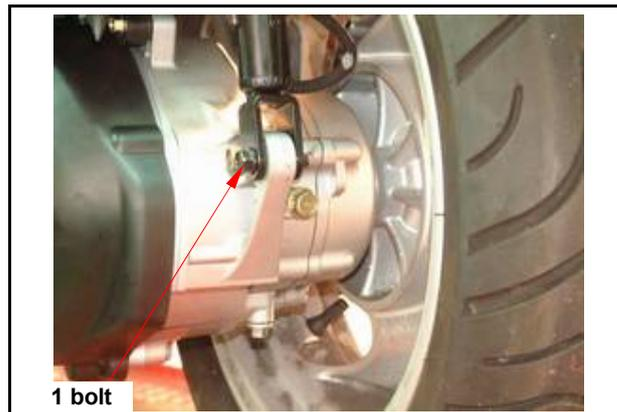
Remove frame side engine hanger bolts (each side 1 bolt), and then remove engine.
