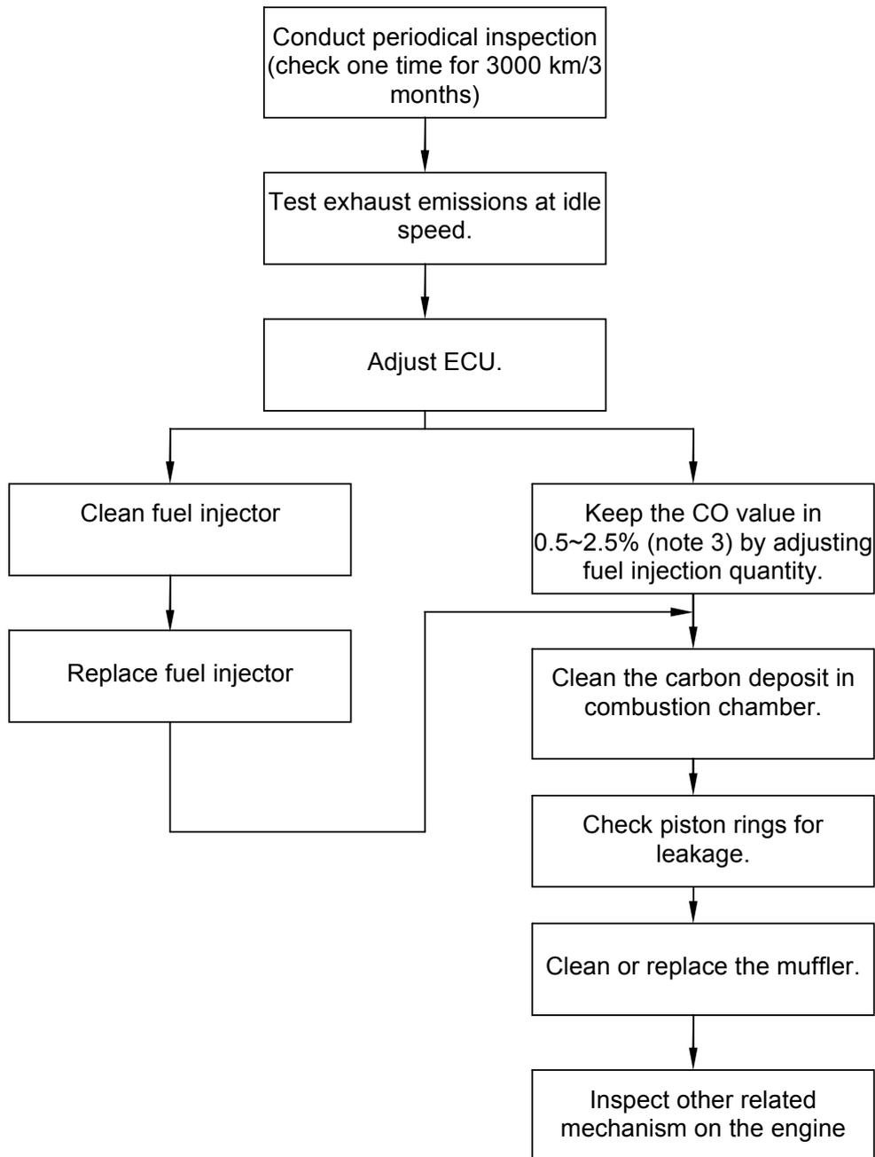
Note: If CO value can not be adjusted to the default value by adjusting ECU, follow the procedures to check or replace components.
