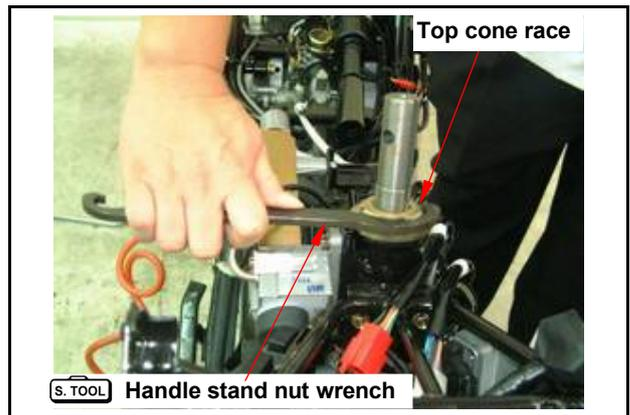
Slightly tap the top and bottom ball bearing seats with a plastic hammer to remove the seats.
