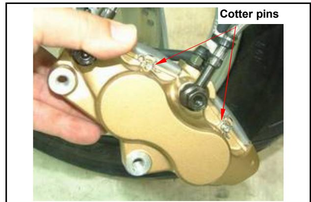
Remove the brake pad shafts and pads.
