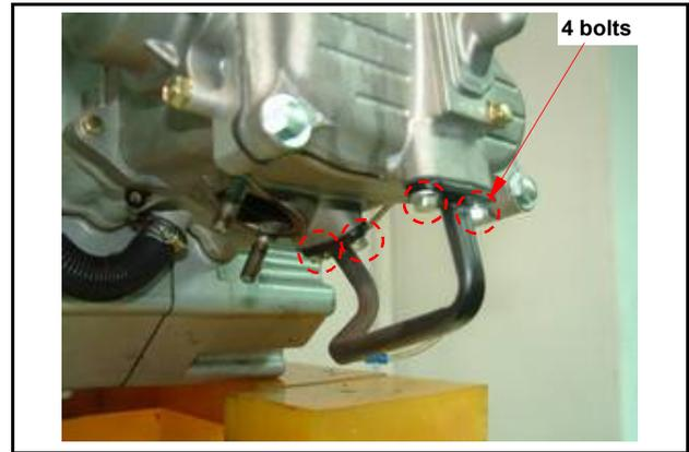
Remove the cylinder head side cover.
