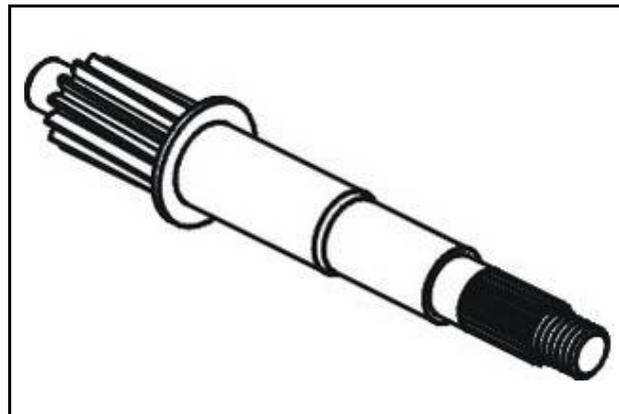
Check if the countershaft is worn or damaged, replace it if necessary.
