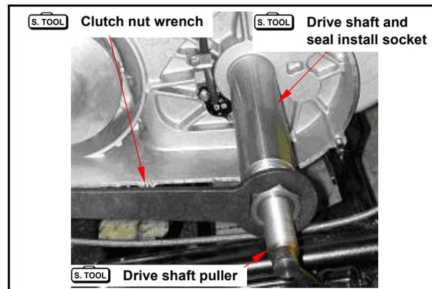
Apply with grease onto drive shaft oil seal.
