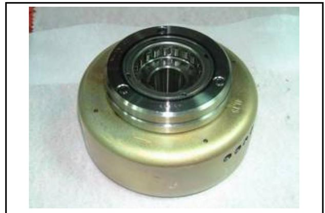
Install starting clutch driven gear onto one way clutch.
