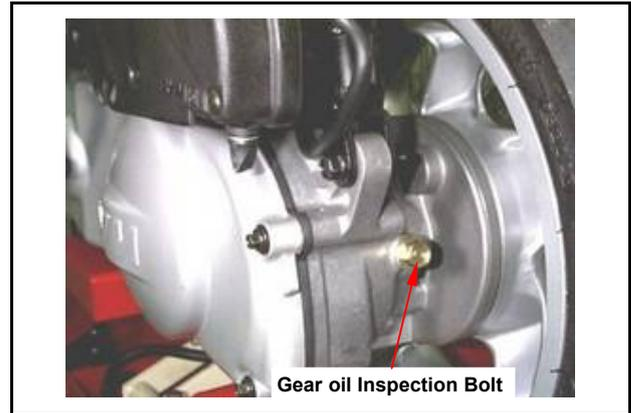
Gear lubrication oil quantity has to be measured with measure device.
