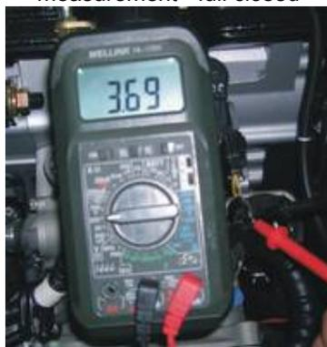
Throttle output signal measurement - full
