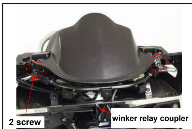
Remove the 4 screws from the handle lower cover rear side.
