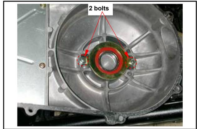
Check bearing on left crankcase cover. Rotate bearing's inner ring with fingers. Check if bearings can be turned in smooth and silent, and also check if bearing outer ring is mounted on cover tightly. If bearing rotation is uneven, noising, or loose bearing mounted, then replace it.
