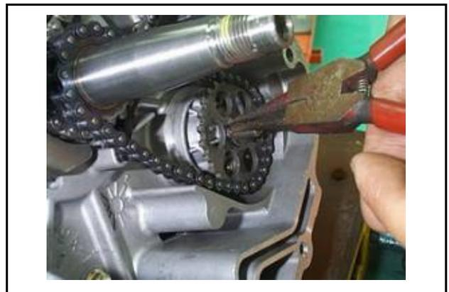
Install starting gear and generator.
