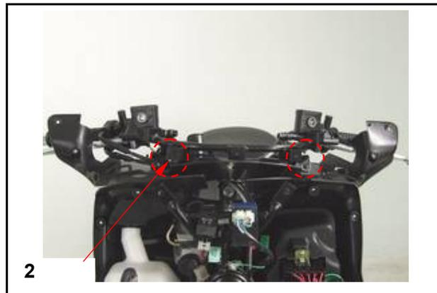
Remove the handle stand nut and bolt.
