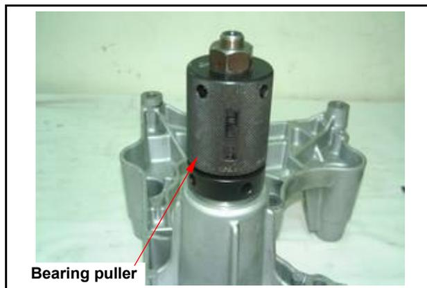
Use screw driver holder bearing puller lower part, and turn the bearing puller upper part to install the rear fork bearing.
