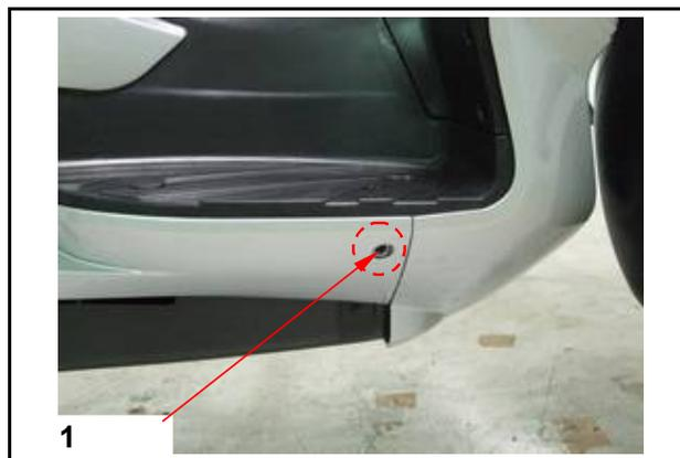
Loosen 1 screw from left and right side for side covers rear upper side.
