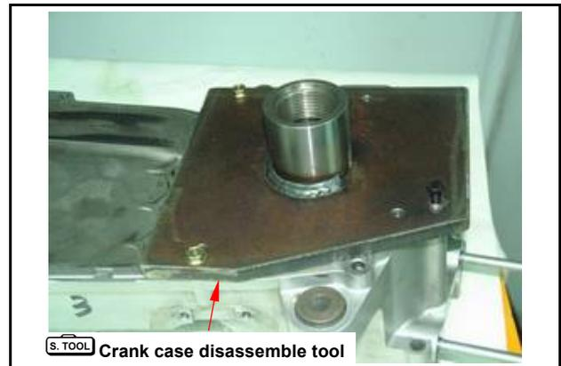
Install left crank shaft puller into crank case disassemble.
