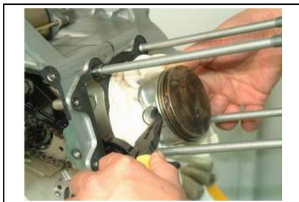
Remove cylinder gasket and dowel pin.
