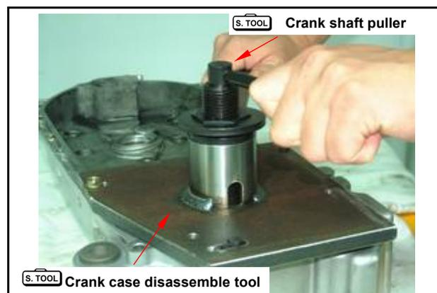
Install crank shaft onto the left crankcase and install crank shaft install socket.
