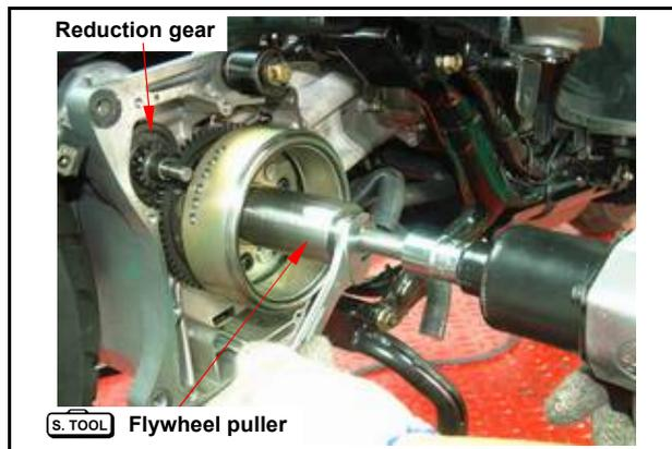
Remove flywheel and starting driven gear.
