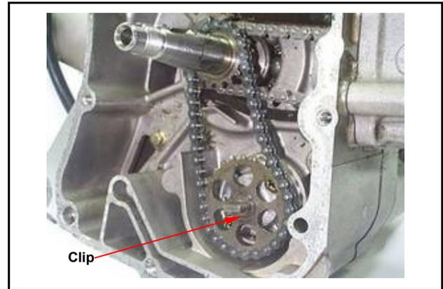
Make sure that pump shaft can be rotated freely. Remove 2 bolts on the oil pump, and then remove oil pump.
