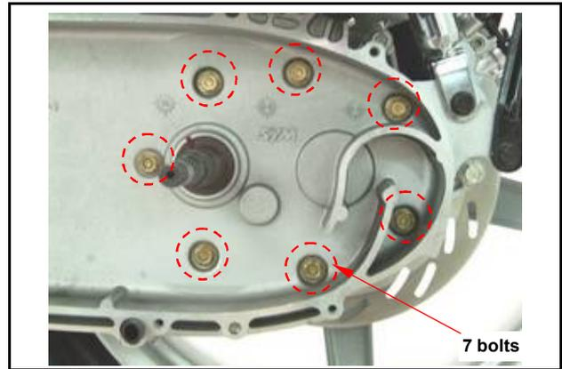
Remove the gear box cover.
