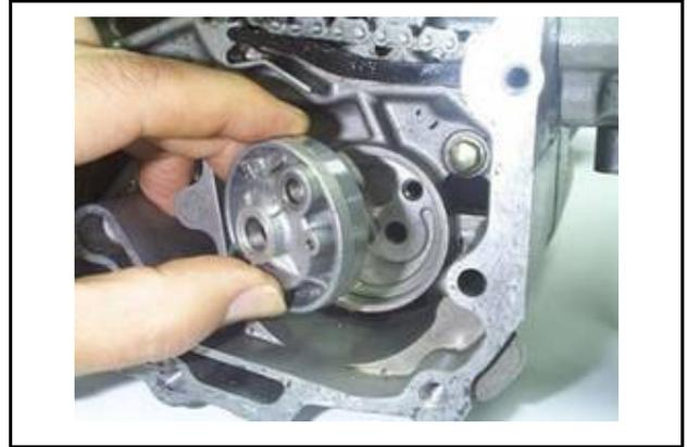
Make sure that oil pump shaft can be rotated freely.
