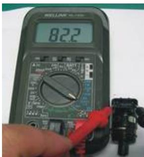
A phase measurement of the resistance value
