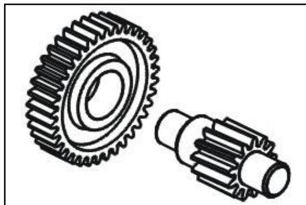
Check if the final shaft and gear are worn or damaged, replace it if necessary.
