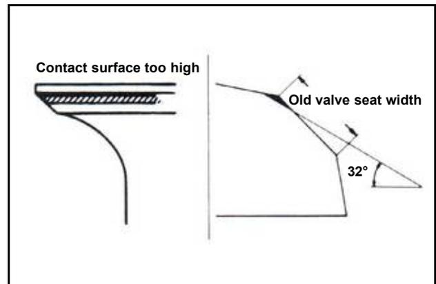
If the contact surface is too high, grind the valve seat with 32° cutter.
