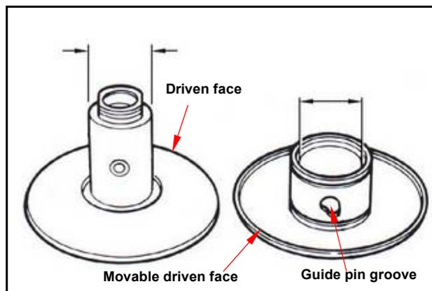
**Driven Pulley Bearing Inspection**
