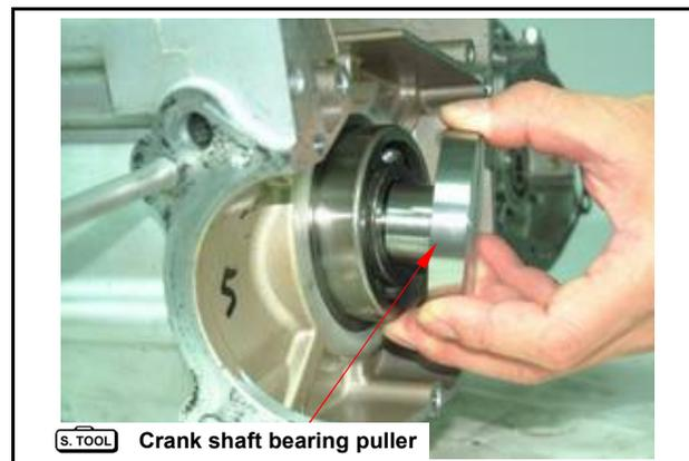
Install crank disassemble tool onto left crankcase. Install left crank shaft puller into crank case disassemble.
