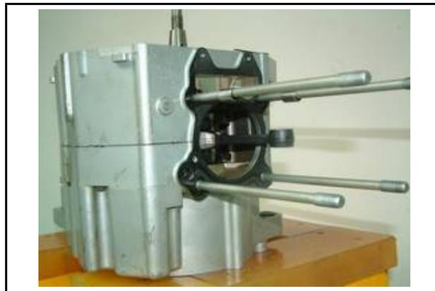
Tighten 8 bolts on the left crankcase.
