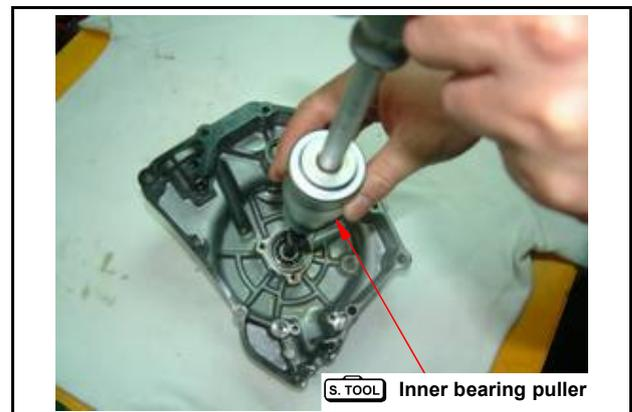
Install the bearing 6201 bearing with special tool.
