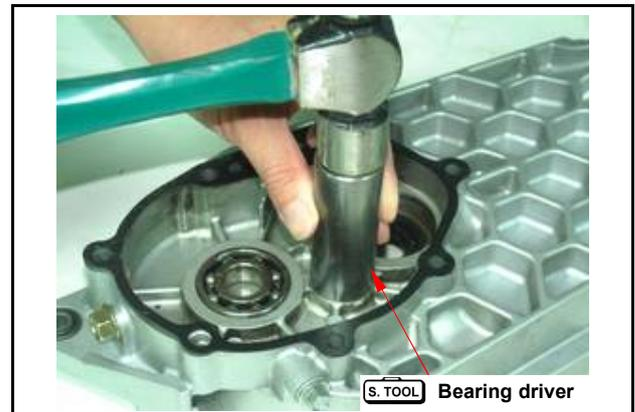
Install new drive shaft bearing and bearing puller onto left crankcase.
