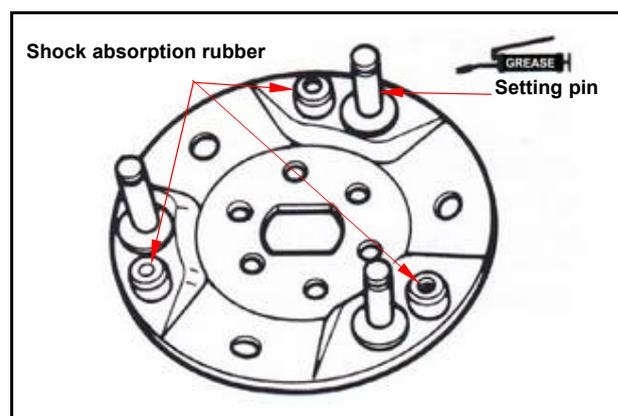
Install new clutch weight onto setting pin and then push to the specified location. Apply with grease onto setting pins. But, the clutch block should not be greased. If so, replace it.
