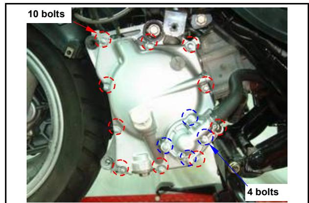
Connect coolant hoses onto the right crankcase cover.
