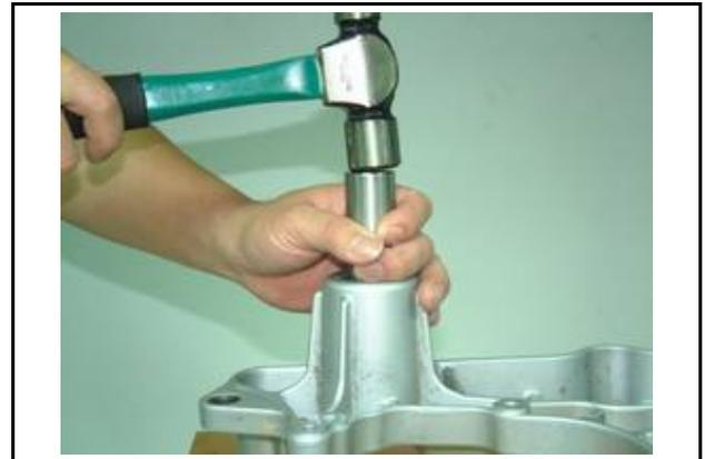
Install new rear fork bearing and bearing puller (6303) onto rear fork.
