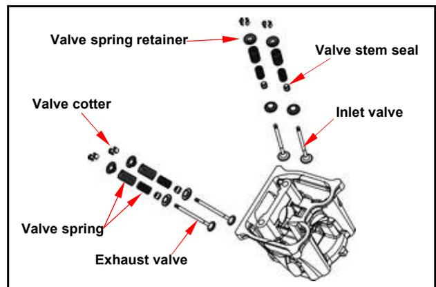
Put the valve coppers onto valve spring retainer.
