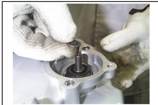
Install the rotor onto the water pump shaft and tighten.
