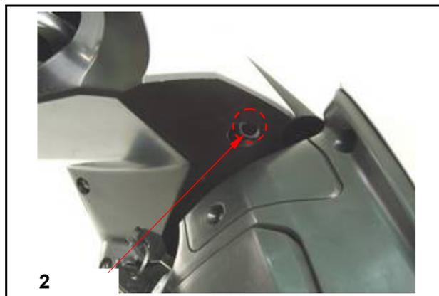
Loosen 2 screws from left and right side for handle front cover after side
