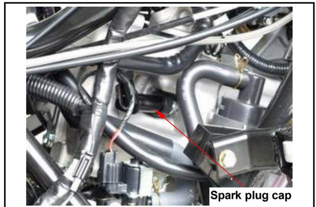
Loosen 2 bolts and replace the ignition coil if necessary.
