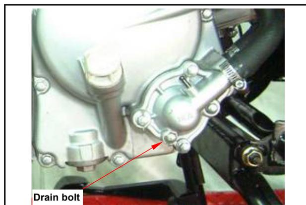
Refill system with the coolant and bleed out the air bubbles.
