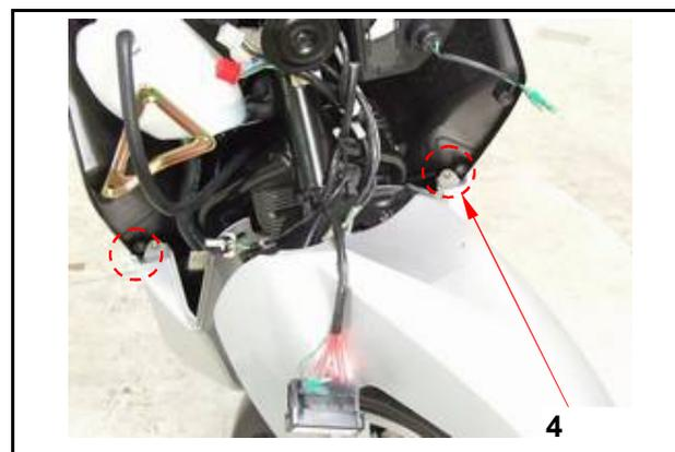
Disassemble the headlight coupler
