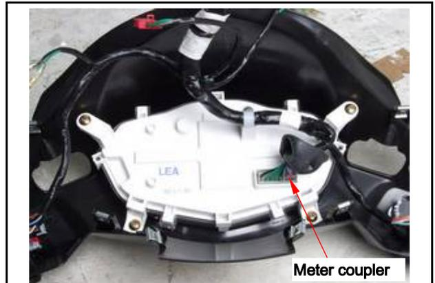
Loosen 4 screws from meter panel.
