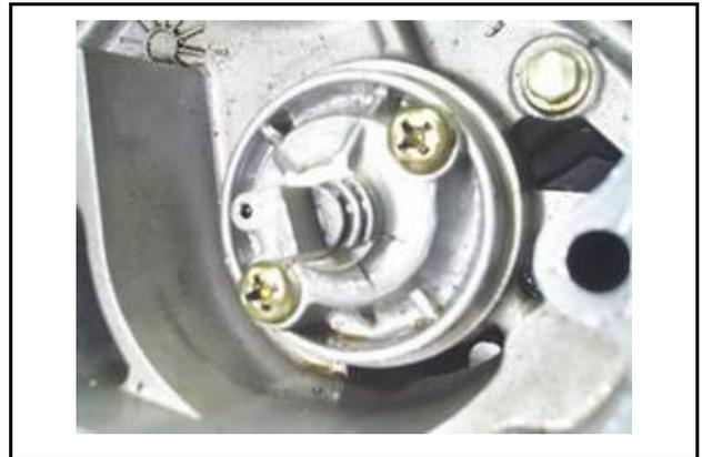
Install oil pump driving chain and sprocket, and then install snap ring onto oil pump shaft.
