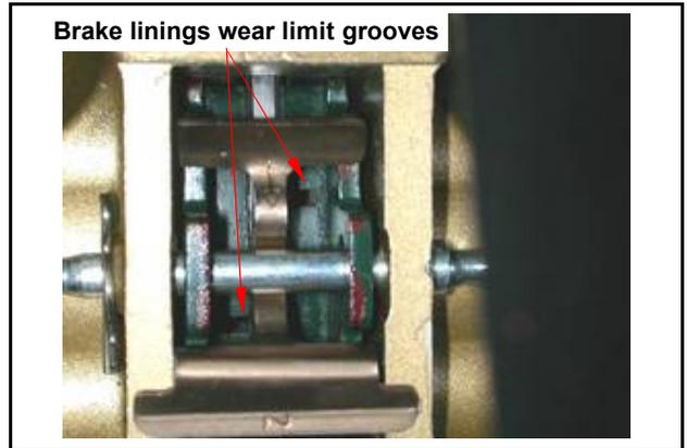
The brake pad must be replaced with new lining when the brake pad wear limit reaches the brake disk.
