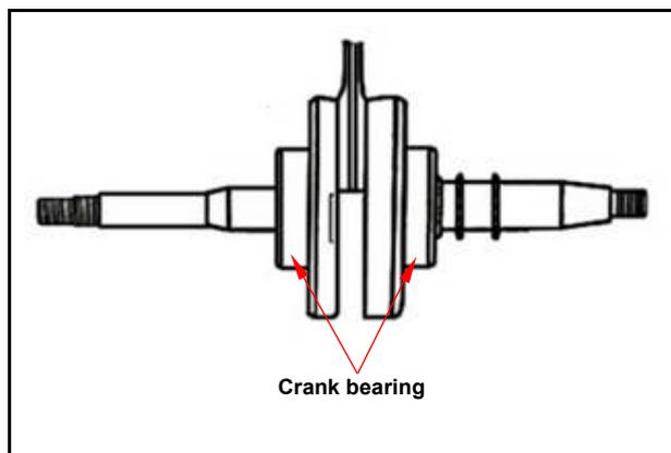
If any roughness, noise and loose linkage are detected, replace the bearing with new one.
