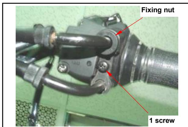
Loosen 2 screws from the throttle holder.
