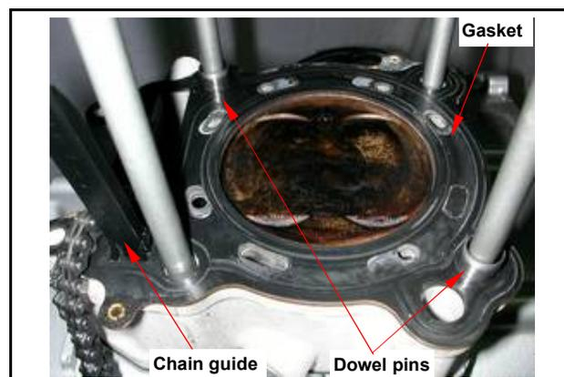
Install 4 washers and tighten 4 nuts on the cylinder head upper side, and then tighten 2 cylinder head mounting bolts of cylinder head right side.
