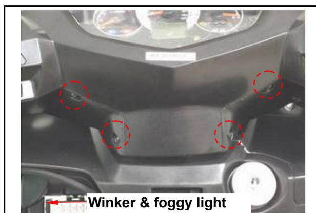
Disassemble the winker relay and brake light couplers
