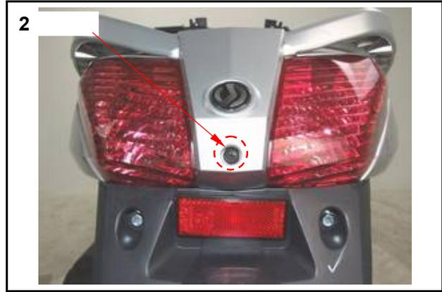
Loosen 2 bolts front tail light upper side.
