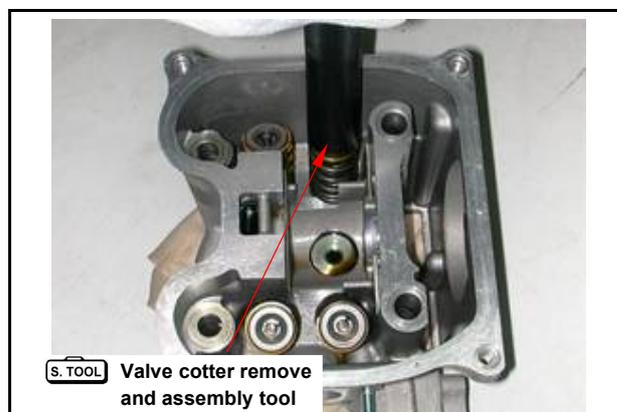
Remove valve cotters, spring retainers, springs and valves.
