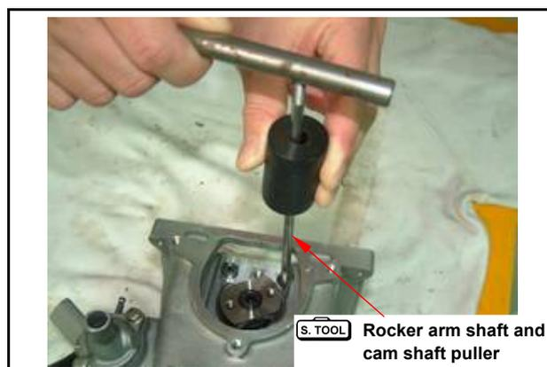
Remove cam shafts.
