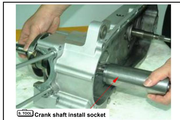
Turn in the crank shaft puller spiral tooth to the left crank shaft.
