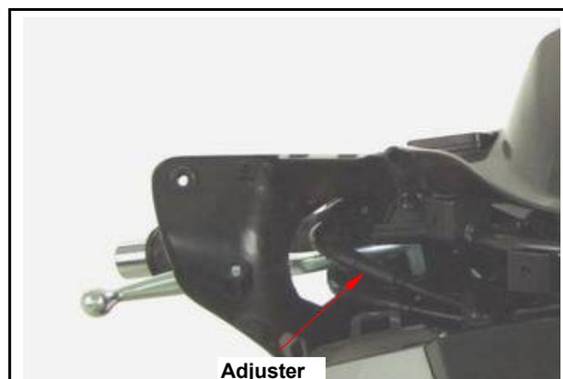
Primary adjustment should be carried out from bottom end of the throttle cable.
