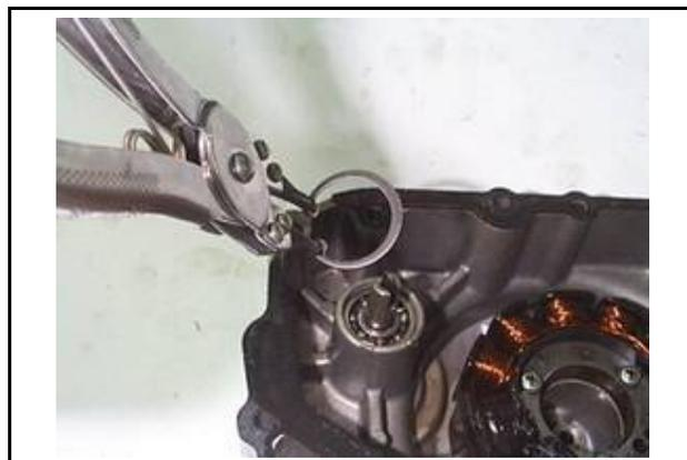
Install the seal washer into the rotor.
