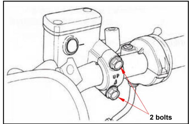
Connect brake hoses with 2 new washers. Tighten the brake hose bolt to the specified torque value. Make sure the hose is installed correctly. Install all wires, hoses, and components carefully so avoid to twisting them together.
