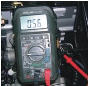
Throttle output signal measurement - full closed
