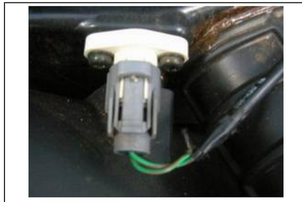
Remove intake tube fixed bolt (bolt×1).
