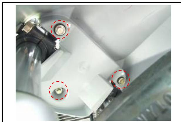
Loosen 2 screws from the front fender above the inside
