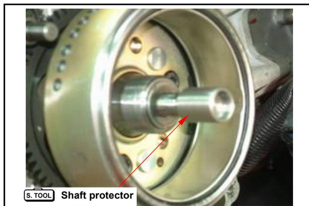
Remove starter reduction gear and shaft.
