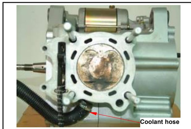
Cover the holes of crankcase and cam chain with a piece of cloth.
