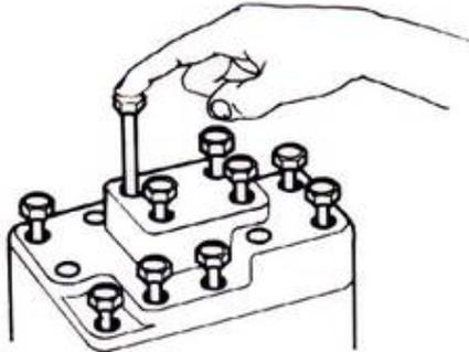
Tighten assemblies with different dimension fasteners as follows: Tighten all the fasteners with fingers, then tighten the big ones with special tool first diagonally from inside toward outside, important components should be tightened 2 to 3 times with appropriate increments to avoid warp unless otherwise indicated. Bolts and fasteners should be kept clean and dry. Do not apply oil to the threads.
