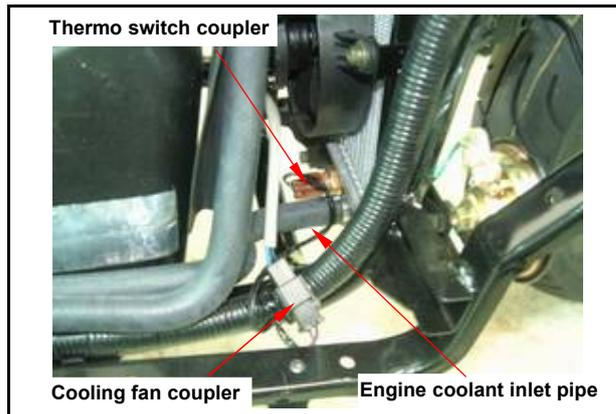
Remove reserve tank coolant inlet pipe.
