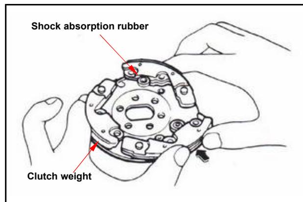
Install the spring into groove with pliers.
