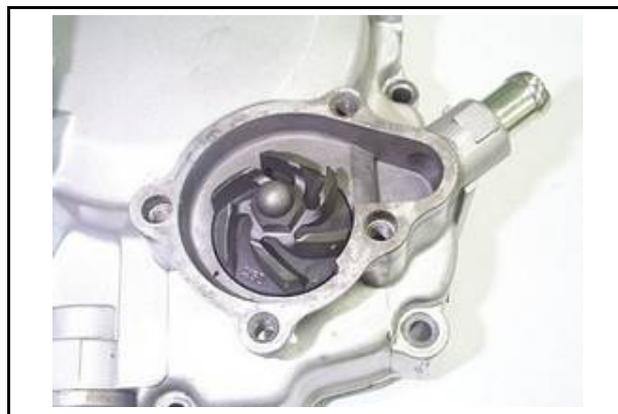
Install the dowel pin and new gasket. Install the water pump cover with 4 bolts.
