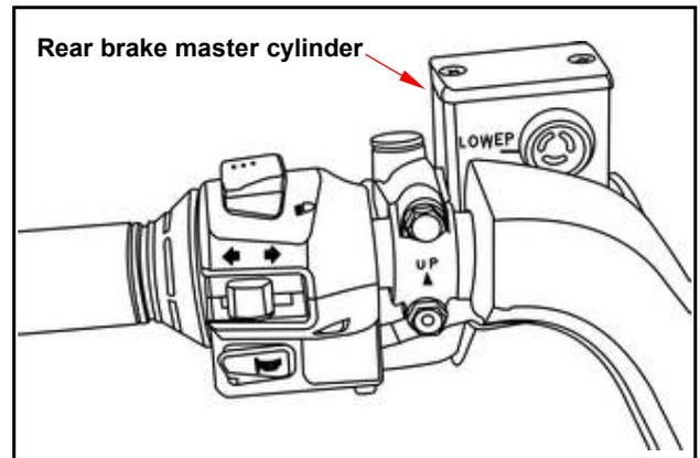
Remove the master cylinder cap and diaphragm. Increases the high quality brake fluid, uses by all means must with the trade mark brake fluid joins in the master cylinder.
