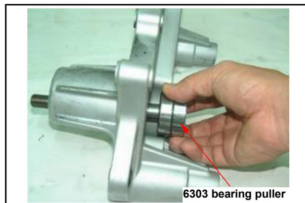
Install the washer of the 6303 bearing puller.
