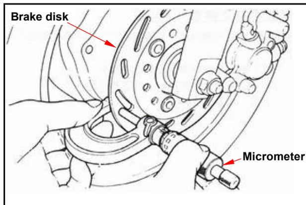
Remove the brake disk from wheel. Check the disk for deformation and bend.
