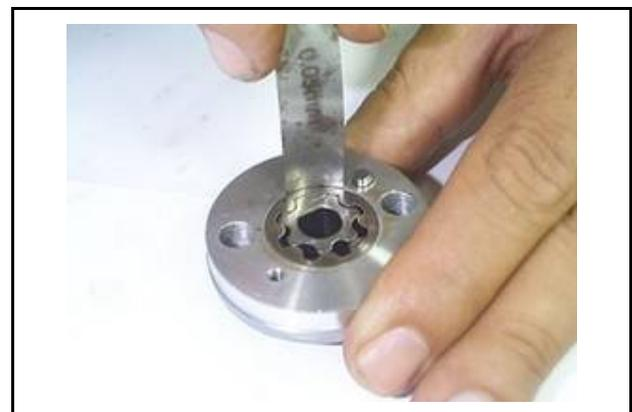
Check clearance between inner and outer rotors.
