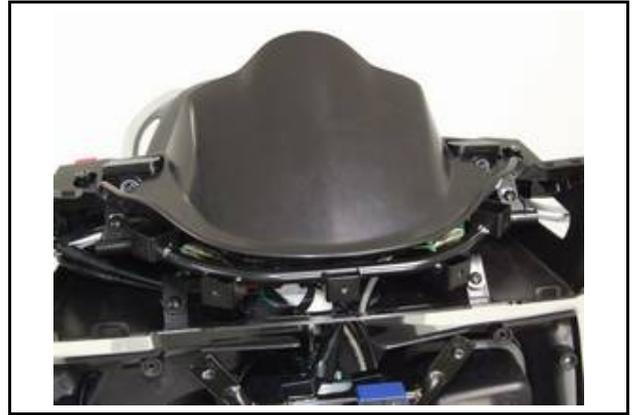
Disconnect the coupler of the speedometer, and take off the meter.
