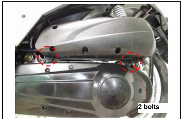
Loosen the 3 bolts from muffler.
