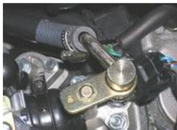
Fuel pressure measurement demolition - injector
