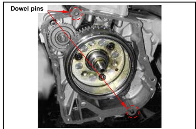
Install right crankcase cover (10 screws).
