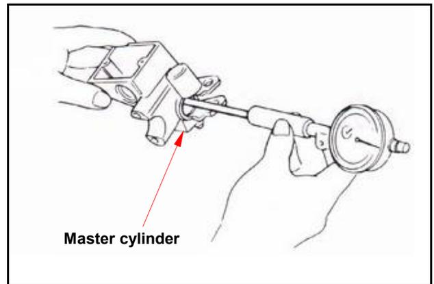
Measure the outer diameter of the piston.
