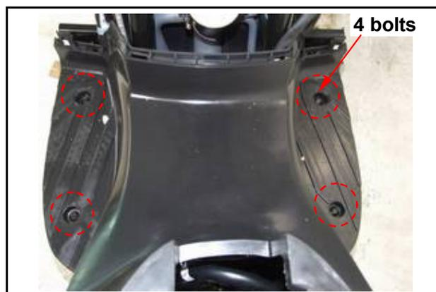
Loosen each side 1 screws from floor panel rear side.
