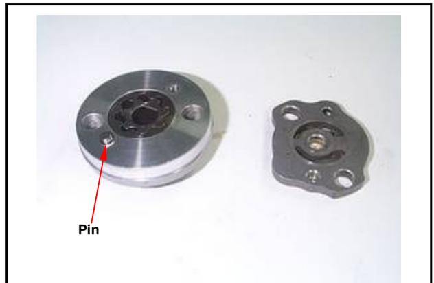
Install the oil pump cover and fixing pin properly
