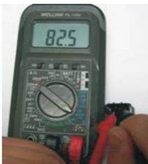
B phase measurement of the resistance value
