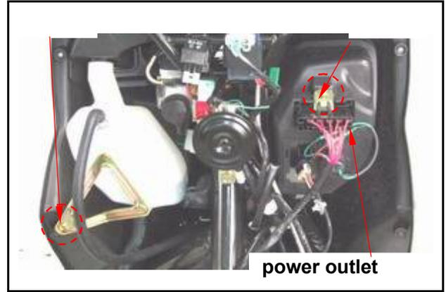
Remove main switch cap bolt then remove main switch cap.
