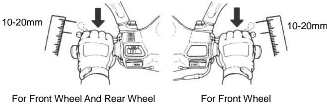
§DISK BRAKE INSPECTION§(Applicable for model equipped with disc brake.)
